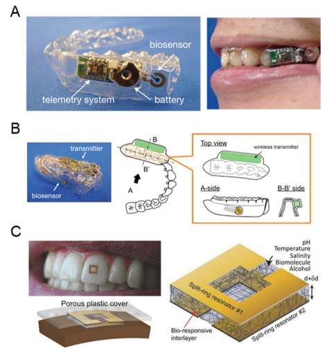
Fig. 6 Saliva-based glucose sensor. (A) Wearable device for saliva glucose estimation (reprinted with permission from ref. 101. Copyright 2020 American Chemical Society), (B) mouthquard biosensor with telemetry system for glucose monitoring (reprinted with permission from ref. 102. Copyright 2016 Elsevier.), (C) wearable sensor on human teeth for the detection of biomolecules (reprinted with permission from ref. 103. Copyright 2018 Wiley-VCH Verlag GmbH & Co).
