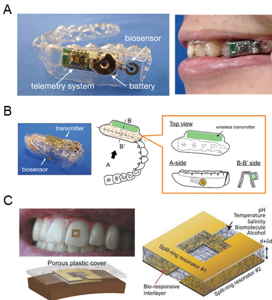
**Fig. 6** Saliva-based glucose sensor. (A) Wearable device for saliva glucose estimation (reprinted with permission from ref. 101. Copyright 2020 American Chemical Society), (B) mouthguard biosensor with telemetry system for glucose monitoring (reprinted with permission from ref. 102. Copyright 2016 Elsevier.), (C) wearable sensor on human teeth for the detection of biomolecules (reprinted with permission from ref. 103. Copyright 2018 Wiley-VCH Verlag GmbH & Co).
