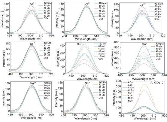
Fig. 5 Fluorescence spectra of Ai-CDs-2 with different concentrations of metal ions, such as Al<sup>3+</sup>, Cd<sup>2+</sup>, Mn<sup>2+</sup>, Ni<sup>2+</sup>, Co<sup>+2</sup>, Cu<sup>+</sup>, and As<sup>+3</sup>, at concentrations of 0, 10, 20, 40, 60, 80, and 120  $\mu M$ .
