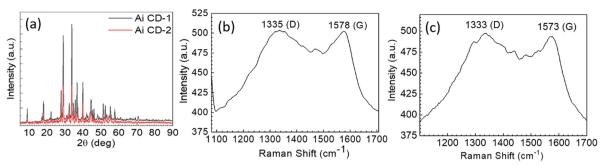
Fig. 3 (a) The XRD pattern of synthesized carbon dots Ai-CDs-1 and Ai-CDs-2, and (b and c) Raman spectroscopic analysis of Ai-CDs-1 and Ai-CDs-2, respectively.
