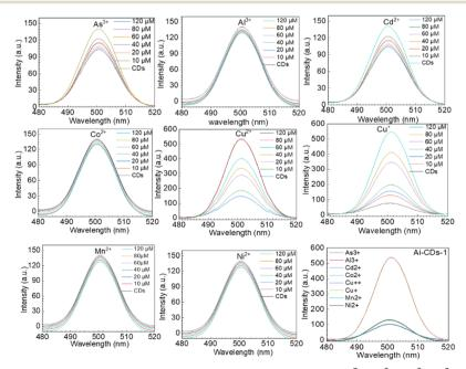
Fig. 4 Fluorescence spectra of Ai-CDs-1 with different concentrations of metal ions, such as Al<sup>3+</sup>, Cd<sup>2+</sup>, Mn<sup>2+</sup>, Ni<sup>2+</sup>, Co<sup>+2</sup>, Cu<sup>+</sup>, Cu<sup>+</sup>, and As<sup>+3</sup>, at different concentrations, such as 0, 10, 20, 40, 60, 80, and 120  $\mu M$
