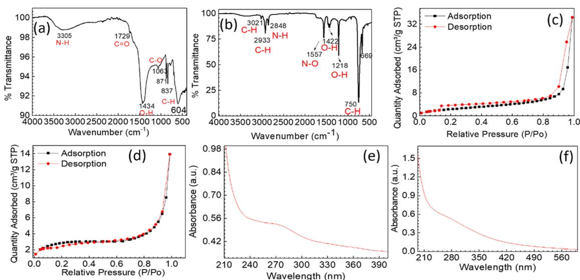
**Fig. 2** (a and b) FTIR spectra of Ai-CDs-1 and Ai-CDs-2, (c and d) BET  $N_2$ -adsorption-desorption isotherms for Ai-CDs-1 and Ai-CDs-2, (e and f) UV-vis spectra for Ai-CDs-1 and Ai-CDs-2, respectively.
