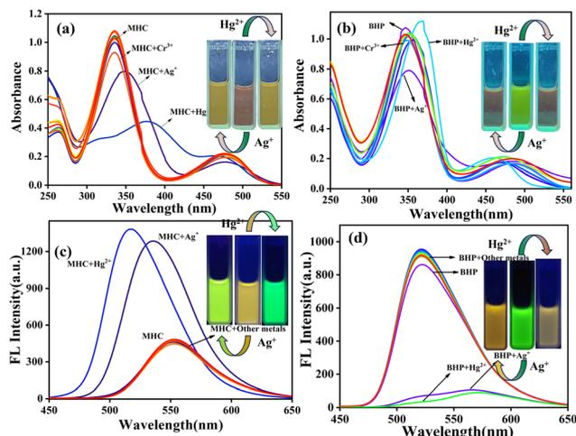
**Fig. 3** UV-visible absorbance selectivity spectra of the sensors (a) **MHC**, (b) **BHP** and fluorescence emission selectivity spectra of (c) **MHC** and (d) **BHP** in the presence of various metal ions ( $1 \times 10^{-3}$  M, 10 equivalents) in ACN:H<sub>2</sub>O (8:2) solutions. The addition of Ag<sup>+</sup> and Hg<sup>2+</sup> ions caused noticeable naked-eye color changes in **MHC** and **BHP**, as shown in (a) and (b), along with fluorescence color changes depicted in (c) and (d).
