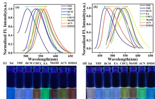
**Fig. 1** (a and b) Normalized fluorescence spectra of the solutions of **MHC** and **BHP** in different solvents (non-polar to polar). (c and d) Fluorescence bottle images of **MHC** and **BHP** under portable UV light radiation (365 nm) in various solvents, such as Tol – toluene; THF – tetrahydrofuran; DCM – dichloromethane; EA – ethyl acetate; CHCl<sub>3</sub> – chloroform; MeOH – methanol; ACN – acetonitrile; DMSO – dimethyl sulfoxide.
