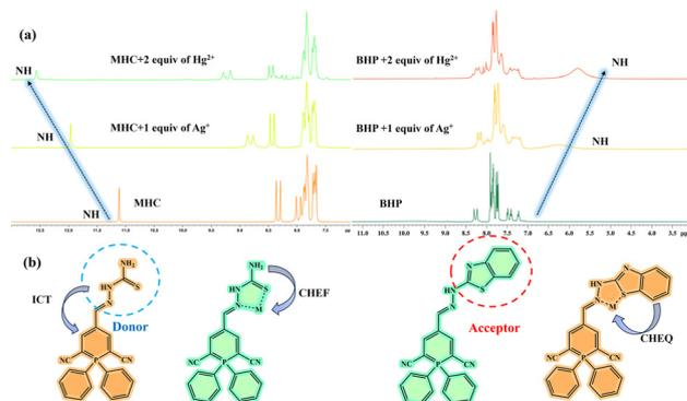
**Fig. 5**  $^1\text{H}$  NMR titration spectra of **MHC** and **BHP** after additions of  $\text{Ag}^+$  and  $\text{Hg}^{2+}$  ions (0–2 equivalents) in  $\text{DMSO}-d_6$ . (b) Chemical structures of **MHC**, **BHP** and its complexes with  $\text{Ag}^+$  and  $\text{Hg}^{2+}$  ions.
