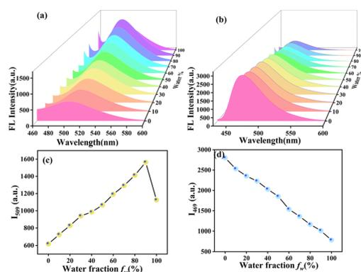
**Fig. 2** (a and b) 3D fluorescence emission spectra of **MHC** and **BHP** ( $2 \times 10^{-5}$  M) in THF/H<sub>2</sub>O (0–100%). (c and d) Plots of  $I_{509}$  nm and  $I_{469}$  values versus water fraction% of the solvent system in **MHC** and **BHP**.
