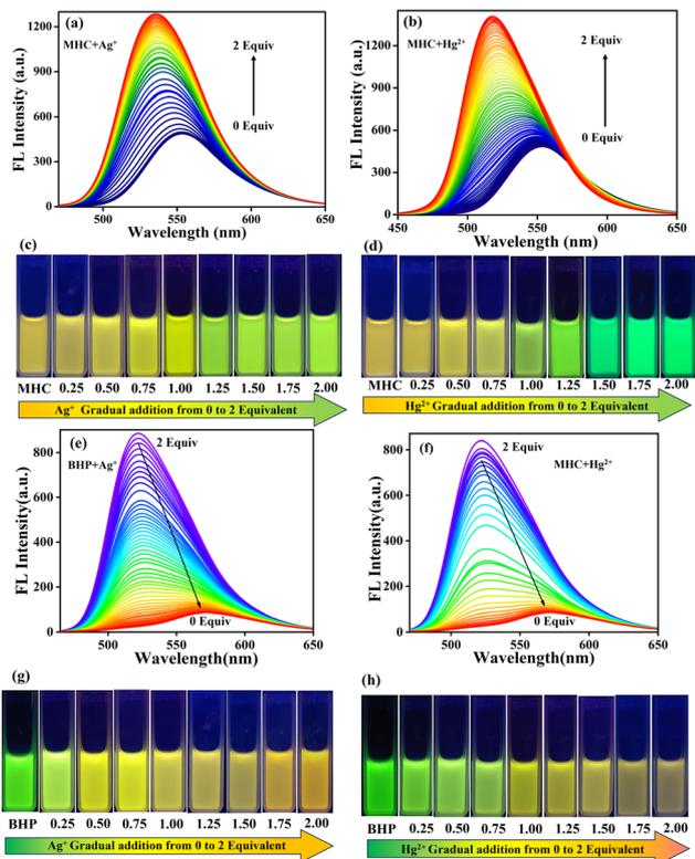
**Fig. 4** Fluorescence emission titration spectra of **MHC** (a and b) and **BHP** (e and f) ( $2 \times 10^{-5}$  M) with the gradual addition of  $\text{Ag}^+$  and  $\text{Hg}^{2+}$  ions in  $\text{ACN}:\text{H}_2\text{O}$  (8:2) solution (0–2 equivalents). The gradual addition of  $\text{Ag}^+$  ions (0–2 equivalents) (c and g) and  $\text{Hg}^{2+}$  ions (0–2 equivalents) (d and h) was performed under a UV lamp emitting at 365 nm.
