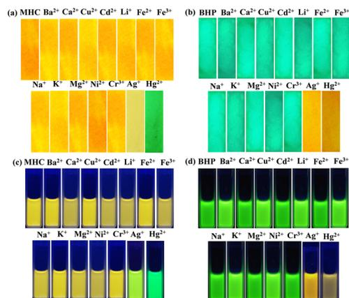
Fig. 6 Image demonstrating the (a) **MHC** and (b) **BHP** fluorescence colour changes that result from adding different metal ions to test paper strips at 365 nm. (b) and (d) Bottle images of **MHC** and **BHP** in the presence of the aforementioned metal ions.
