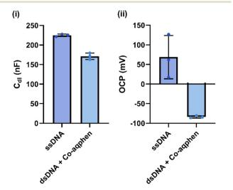
Fig. 4 Data for co-incubation of target DNA and [Co(GA)2(agphen)]Cl intercalator showing the response of simultaneous hybridization and intercalation on (i) capacitance, and (ii) OCP in 100 mM PB ( $n \ge 3$ ).
