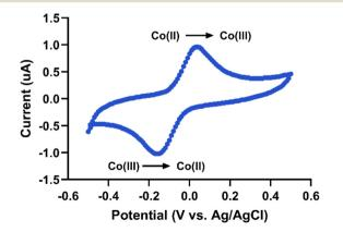
Fig. 3 Cyclic voltammogram of dsDNA-bound [Co(GA)2(agphen)]Cl in 100 mM PB at a scan rate of 0.2 V s<sup>-1</sup> vs. Ag/AgCl.
