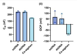
Fig. 2 The responses of DNA hybridization and [Co(GA)2(aqphen)]Cl intercalation on non-faradaic EIS measurements in 100 mM PB. (i) Double-layer capacitance response. (ii) Response of the open circuit potential (OCP) ( $n \ge 3$ ).
