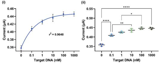
Fig. 6 Differential pulse voltammetry current response to the binding of ssDNA and [Co(GA)<sub>2</sub>(aqphen)]Cl. (i) Dose-response curve for detection between 0.1–1000 nM E. coli ssDNA in 100 mM PB (n ≥ 3). (ii) The results of an ordinary one-way ANOVA related to the dose-response of E. coli ssDNA between 0.1–1000 nM ( $n \ge 3$ ).
