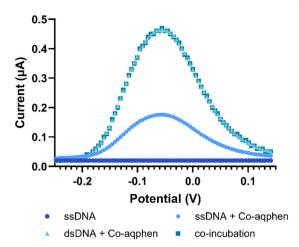
Fig. 5 Differential pulse voltammograms after co-incubation with target DNA and [Co(GA)<sub>2</sub>(aqphen)]Cl in 100 mM PB at a scan rate of 50 mV s<sup>-1</sup> vs. Ag/AgCl.
