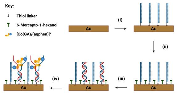
Scheme 3 Design and fabrication of the DNA sensor and assay steps for detection of E. coli ssDNA. (i) Incubation in a 1:10 solution of HS-(CH)<sub>6</sub>ssDNA and MCH overnight. (ii) Backfilling with MCH to fill pinholes. (iii) Hybridization with target ssDNA to form surface-bound dsDNA. (iv) [Co(GA)2(aqphen)]Cl was incubated and intercalated with dsDNA, causing unwinding of the dsDNA helix structure.
