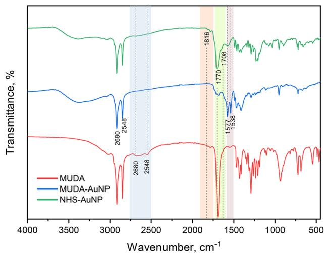
**Fig. 4** FTIR spectra of MUDA (11-mercaptopundecanoic acid), MUDA-AuNP, and NHS-AuNP (NHS functionalized - MUDA-AuNP). The difference in the highlighted FT-IR peaks suggests successful MUDA functionalization and subsequent NHS-MUDA formation.
