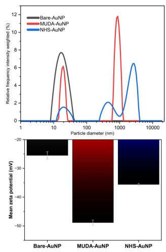
Fig. 5 (Up) Particle size distribution of bare-AuNP, MUDA-AuNP (11mercaptoundecanoic acid functionalized AuNP), and NHS-AuNP (NHS/ EDC activated MUDA-AuNP). Their hydrodynamic sizes (dhydro) are 17.26 nm, 493 nm, and 2167 nm, respectively. (Down) ζ-Potential of bare-AuNP, MUDA-AuNP, and NHS-AuNP are -25.50 mV, -48.86 mV, -35.59 mV, respectively. The shifts in particle sizes and  $\zeta$ -potential suggest successful functionalization and subsequent NHS-AuNP formation.
