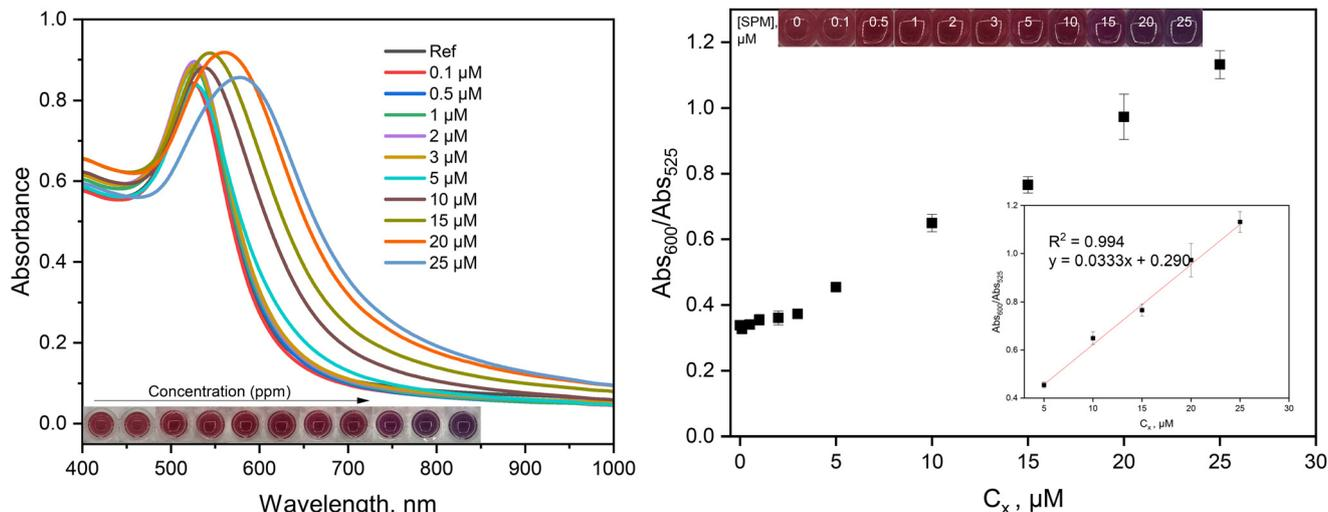
Fig. 7 (Left) Absorption spectra of MUDA-AuNP (11-mercaptopundecanoic acid functionalized AuNP) with increasing spermine concentration (0–25  $\mu\text{M}$ ). (Right) Corresponding absorption ratios of MUDA-AuNP plotted against increasing spermine concentration. At a specific range (5–25  $\mu\text{M}$ ), MUDA-AuNP absorption ratios linearly increase with increasing spermine concentration in the solutions. Inset: Actual images of the solutions.
