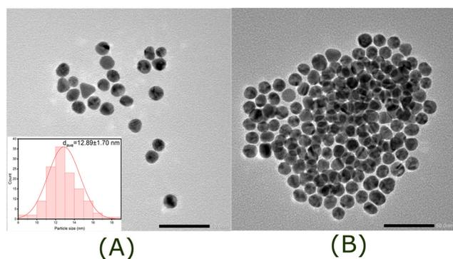
**Fig. 2** TEM image of (A) MUDA-AuNP (11-mercaptoundecanoic acid functionalized AuNP) and (B) MUDA-AuNP in the presence of  $19 \mu\text{M}$  spermine. With MUDA functionalization, the particle size slightly increased ( $12.9$  nm to  $13.8$  nm), and superior stability was observed. As shown in B, spermine addition caused AuNP aggregation. Inset: (A) AuNP particle size distribution.
