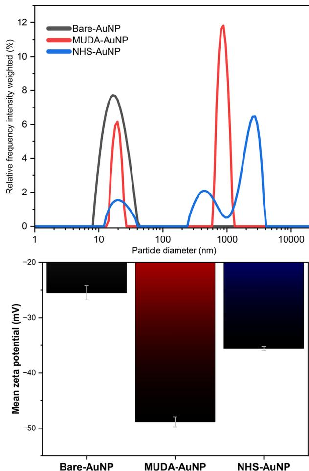
**Fig. 5** (Up) Particle size distribution of bare-AuNP, MUDA-AuNP (11-mercaptopundecanoic acid functionalized AuNP), and NHS-AuNP (NHS/EDC activated MUDA-AuNP). Their hydrodynamic sizes ( $d_{\text{hydro}}$ ) are 17.26 nm, 493 nm, and 2167 nm, respectively. (Down)  $\zeta$ -Potential of bare-AuNP, MUDA-AuNP, and NHS-AuNP are -25.50 mV, -48.86 mV, -35.59 mV, respectively. The shifts in particle sizes and  $\zeta$ -potential suggest successful functionalization and subsequent NHS-AuNP formation.
