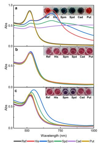
Fig. 6 UV-Vis absorption spectra comparison of a) bare-AuNP, b) MUDA-AuNP (11-mercaptoundecanoic acid functionalized AuNP), and c) NHS-AuNP (NHS-ester conjugated MUDA-AuNP) against 9.5  $\mu$ M of various biogenic amines found in spoiled meat, namely histamine (His), spermine (Spm), spermidine (Spd), cadaverine (Cad), and putrescine (Put). NHS-AuNP shows a selective response towards Spm and Spd compared to other sensors. Inset: Actual images of the solutions.
