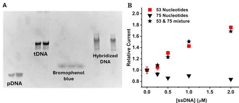
**Fig. 3** A. 14% polyacrylamide gel electrophoresis of 4 μM pDNA, 4 μM tDNA, bromophenol blue dye, and the mixture of the pDNA and tDNA (4 μM final concentration each). B. Response from 53-NT tDNA, 75-NT ssDNA, and mixtures of 53 and 75-NT ssDNA (1:1) from a final concentration of 0.25–2 μM. Error bars represent standard deviation of three replicates and may appear hidden as they are smaller than the size of the data points.
