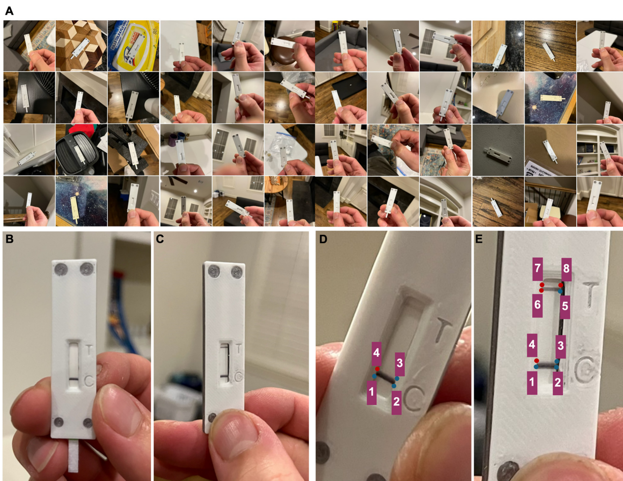
Fig. 1 Smartphone-captured photos of tested LFA devices used to train and validate the ML models. (A) Collage of LFA device photos captured in real-world environments. Representative photos of an LFA device tested on a (B) negative sample and (C) positive sample. The process for manually annotating photos of LFA devices tested on a (D) negative sample and (E) positive sample.
