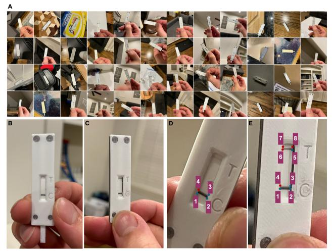
Fig. 1 Smartphone-captured photos of tested LFA devices used to train and validate the ML models. (A) Collage of LFA device photos captured in real-world environments. Representative photos of an LFA device tested on a (B) negative sample and (C) positive sample. The process for manually annotating photos of LFA devices tested on a (D) negative sample and (E) positive sample.
