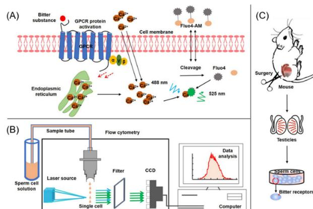
**Fig. 8** (A) Schematic diagram of the detection principle of a cell-based biosensing system; (B) detection principle of the flow cytometry measurement system; (C) process diagram for obtaining mouse sperm cells.<sup>61</sup>
