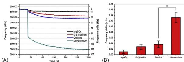
**Fig. 7** (A) Real-time monitoring of crystal resonant frequency shifts indicating responses of a chemical biosensor to MgSO<sub>4</sub>, denatonium, D-(-)-salicin, and quinine. (B) Statistical results of this chemical biosensor with and without bitter receptors responding to different bitter substances.<sup>61</sup>
