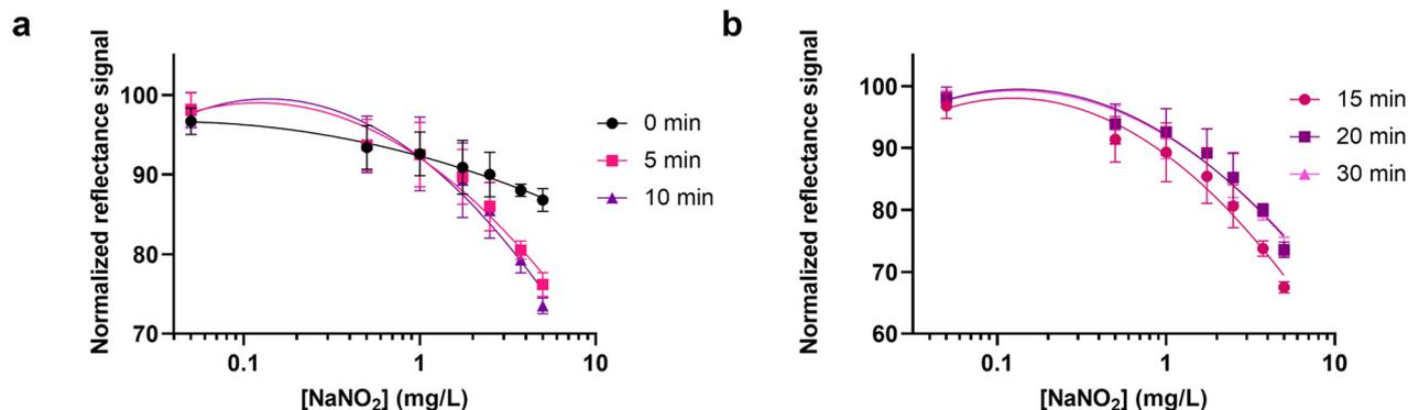
Fig. 2 (a) Calibration curve for  $\text{NaNO}_2$  obtained at 0, 5 and 10 min of incubation in the dark, at RT and (b) at 15, 20 and 30 min acquiring the reflectance signals with the OnePlus 6 smartphone.
