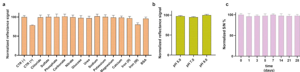
Fig. 4 a) Selectivity studies of the NitriPad with different interferents (2 mM) compared to 2.50 mg L<sup>-1</sup> NaNO<sub>2</sub> (CTR+). Reflectance signals are normalized to the CTR(-), b) pH effects on the NitriPad, and c) stability of the NitriPad stored at +4 °C. Reflectance signals are normalized to day 0.
