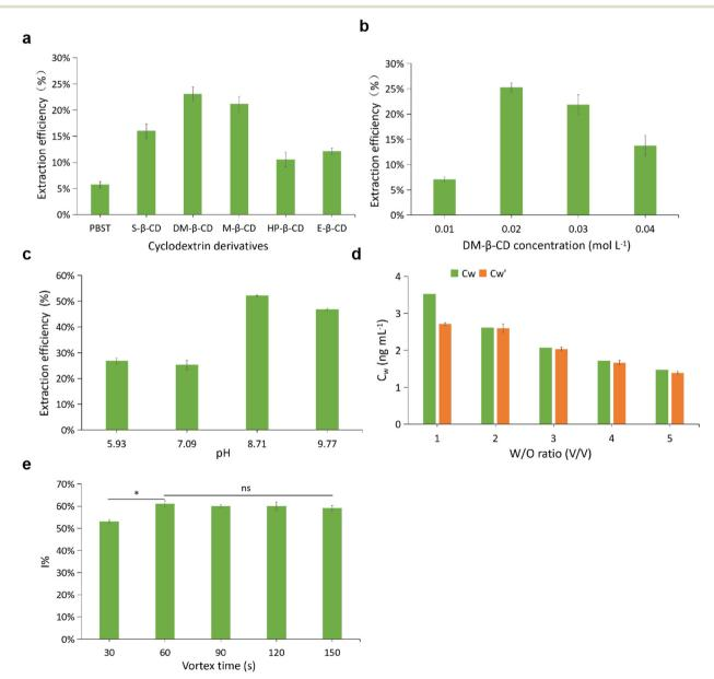
Fig. 2 Optimization of the extraction process. (a) The extraction efficiency of cyclodextrin derivative solutions for capsaicin in oil samples; (b) the extraction efficiency of different DM- $\beta$ -CD concentrations for capsaicin; (c) the effect of pH on the extraction efficiency; (d) the comparation of experimental and theoretical  $C_w$  at different W/O ratios; (e) the effect of shaking time on the l%.
