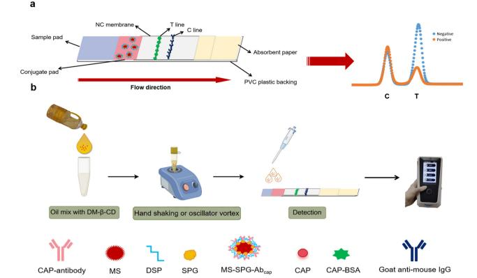
Scheme 1 (a) The structure and detection principle of the LFIA strip. (b) On-site extraction and test process. By Figdraw.
