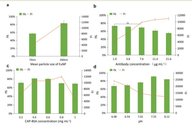
Fig. 1 Optimization of preparation conditions for the LFIA strip for CAP. The effect on the FI values of the T line and the I% when detecting the blank solution and 5 ng mL $^{-1}$  CAP solution (n = 3) by (a) different sizes of EuNPs; (b) different antibody concentrations; (c) different CAP-BSA concentrations; (d) different buffer pH values.
