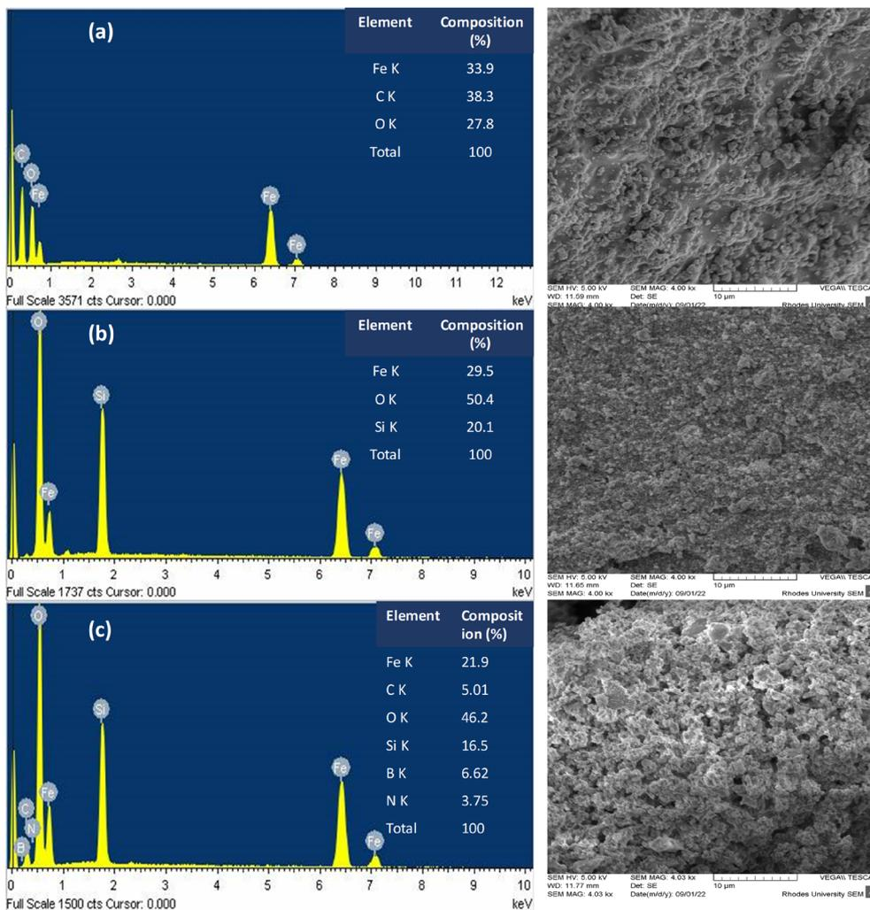
Fig. 3 Energy dispersive X-ray (EDX) spectra with their corresponding SEM images for (a) Fe<sub>3</sub>O<sub>4</sub>NPs, (b) Fe<sub>3</sub>O<sub>4</sub>@SiO<sub>2</sub>NPs, and (c) Fe<sub>3</sub>O<sub>4</sub>@SiO<sub>2</sub>-PBANPs.
