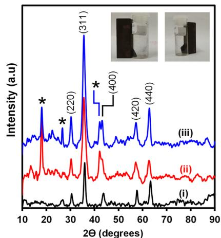
Fig. 1 XRD diffractograms of (i)  $\text{Fe}_3\text{O}_4$ NPs, (ii)  $\text{Fe}_3\text{O}_4@\text{SiO}_2$ NPs, and (iii)  $\text{Fe}_3\text{O}_4@\text{SiO}_2$ -PBANPs. The insert exhibits the photographs of  $\text{Fe}_3\text{O}_4@\text{SiO}_2$ NPs and  $\text{Fe}_3\text{O}_4@\text{SiO}_2$ -PBANPs in the presence of the magnetic field.
