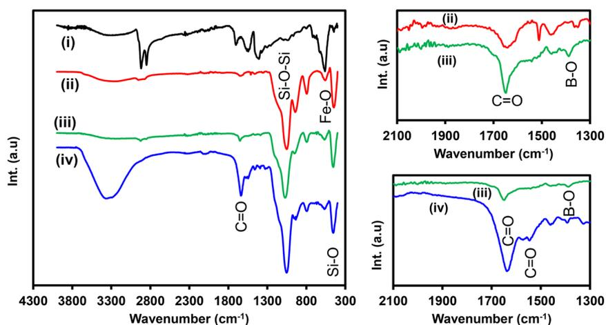
Fig. 4 FT-IR spectra of (i) Fe<sub>3</sub>O<sub>4</sub>NPs, (ii) Fe<sub>3</sub>O<sub>4</sub>@SiO<sub>2</sub>NPs, (iii) Fe<sub>3</sub>O<sub>4</sub>@SiO<sub>2</sub>-PBANPs, and (iv) Fe<sub>3</sub>O<sub>4</sub>@SiO<sub>2</sub>-PBA-Ab<sub>1</sub> (enlarged 1300–2100 cm<sup>-1</sup> for B–O, C=O).
