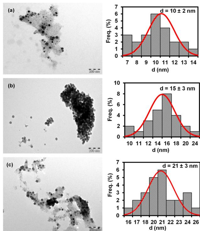
Fig. 2 TEM images and corresponding size distribution histograms of (a)  $\text{Fe}_3\text{O}_4\text{NPs}$ , (b)  $\text{Fe}_3\text{O}_4@\text{SiO}_2\text{NPs}$ , and (c)  $\text{Fe}_3\text{O}_4@\text{SiO}_2\text{-PBANPs}$ .
