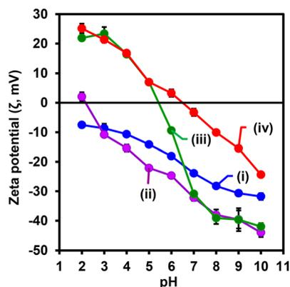
Fig. 5 Zeta potential ( $\zeta$ , mV) vs. pH (2–10, PBS, 10 mM) for (i) Fe<sub>3</sub>O<sub>4</sub>NPs, (ii) Fe<sub>3</sub>O<sub>4</sub>@SiO<sub>2</sub>NPs, (iii) Fe<sub>3</sub>O<sub>4</sub>@SiO<sub>2</sub>-PBANPs, and (iv) Fe<sub>3</sub>O<sub>4</sub>@SiO<sub>2</sub>-PBA-Ab<sub>1</sub>.
