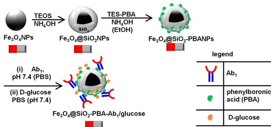
**Scheme 1** Step-by-step preparation of the  $\text{Fe}_3\text{O}_4@(\text{SiO}_2\text{-PBA-Ab}_1/\text{glucose})$  capture nanobioconjugates.
