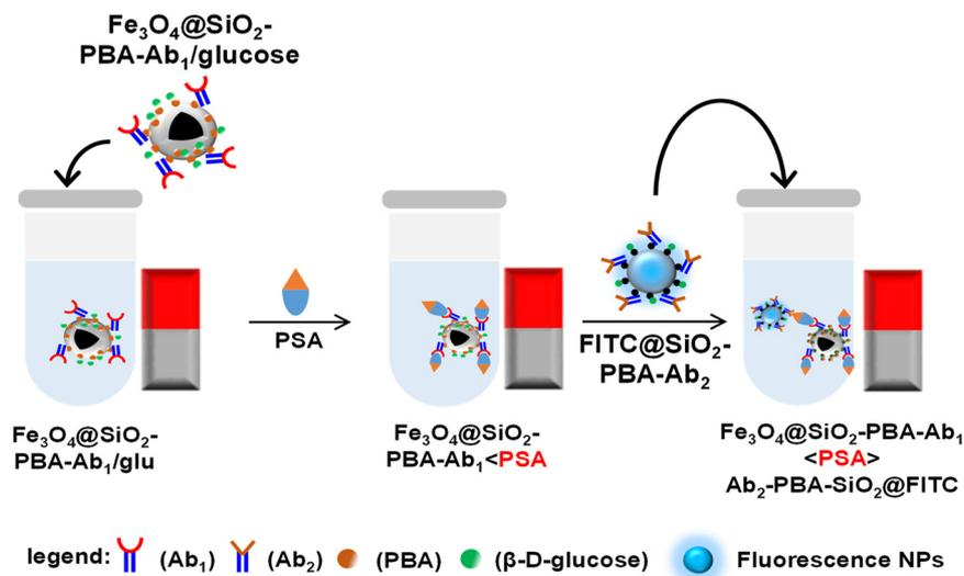
**Scheme 2** Capture of PSA by  $\text{Fe}_3\text{O}_4@\text{SiO}_2\text{-PBA-Ab}_1/\text{glucose}$  and fluorescence detection using  $\text{FITC}@\text{SiO}_2\text{-PBA-Ab}_2/\text{glucose}$ .
