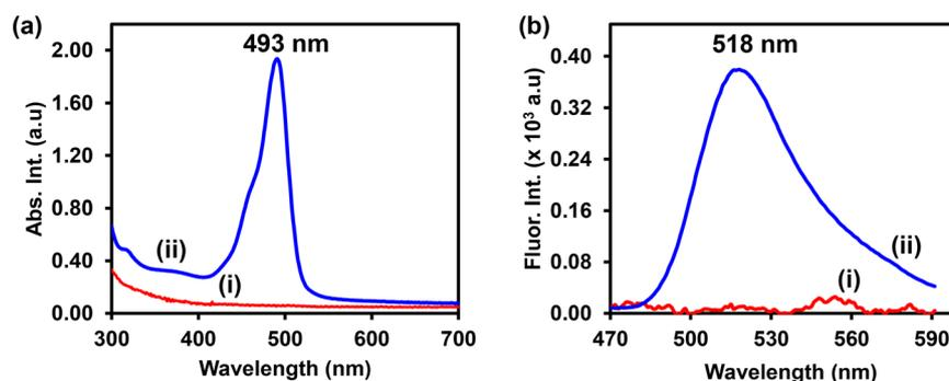
**Fig. 6** (a) UV-vis absorption and (b) fluorescence emission spectra of (i)  $\text{Fe}_3\text{O}_4@\text{SiO}_2\text{-PBA-Ab}_1<\text{PSA}>$ , and (ii)  $\text{Fe}_3\text{O}_4@\text{SiO}_2\text{-PBA-Ab}_1<\text{PSA}>\text{Ab}_2\text{-PSA-FITC}$  sandwich immunoassay.
