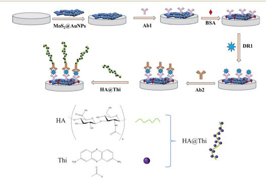
Scheme 1 Scheme diagram of the dual-signal amplification electrochemical biosensor based on MoS<sub>2</sub>@AuNPs and HA@Thi for DR1 detection.
