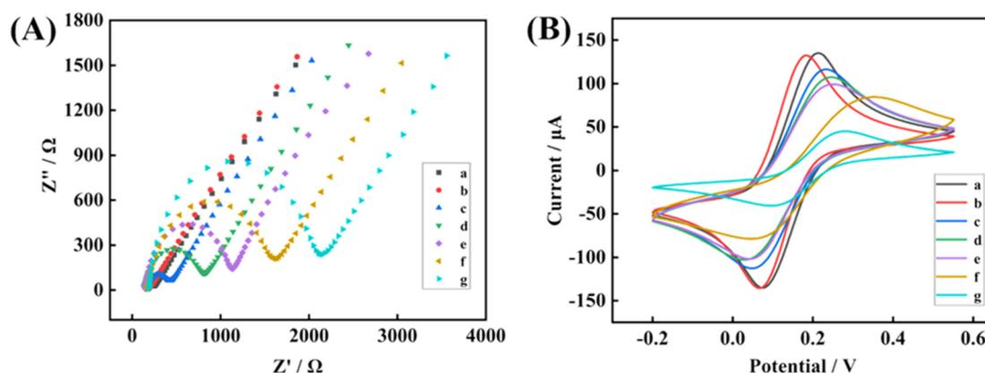
Fig. 3 EIS (A) and CV (B) profiles of layer-by-layer modified electrodes GCE (a),  $\text{MoS}_2\text{@AuNPs}/\text{GCE}$  (b), Ab1/ $\text{MoS}_2\text{@AuNPs}/\text{GCE}$  (c), BSA/Ab1/ $\text{MoS}_2\text{@AuNPs}/\text{GCE}$  (d), DR1/BSA/Ab1/ $\text{MoS}_2\text{@AuNPs}/\text{GCE}$  (e), Ab2/DR1/BSA/Ab1/ $\text{MoS}_2\text{@AuNPs}/\text{GCE}$  (f), and HA@Thi/Ab2/DR1/BSA/Ab1/ $\text{MoS}_2\text{@AuNPs}/\text{GCE}$  (g).
