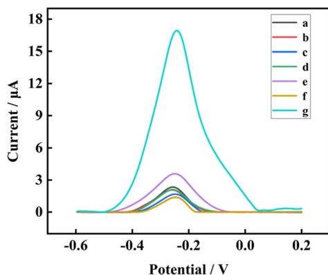
Fig. 2 SWV signal response curves of the electrochemical biosensor after modification with all the components ( $\text{MoS}_2\text{@AuNPs}/\text{Ab1}/\text{DR1}/\text{Ab2}/\text{HA}/\text{Thi}$ ) (g), and without  $\text{MoS}_2\text{@AuNPs}$  (a), Ab1 (b), DR1 (c), Ab2 (d), HA (e), and Thi (f) modification.
