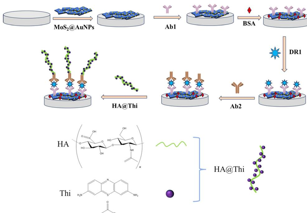
**Scheme 1** Scheme diagram of the dual-signal amplification electrochemical biosensor based on MoS<sub>2</sub>@AuNPs and HA@Thi for DR1 detection.
