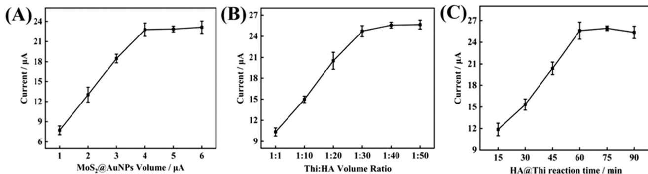
Fig. 4 Effect of (A) the amount of MoS<sub>2</sub>@AuNP nanocomposites, (B) the volume ratio of Thi to HA, and (C) the reaction time of HA@Thi on the peak current (error bars indicate the standard deviation of three replicate parallel experiments, and all DR1 samples were at a concentration of  $1$  ng mL<sup>-1</sup>).
