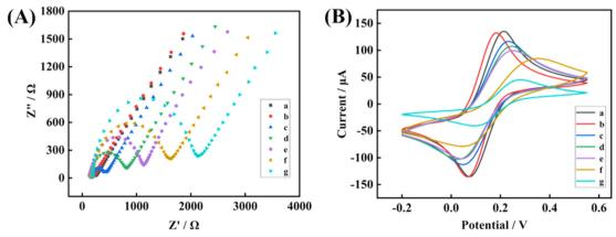
Fig. 3 EIS (A) and CV (B) profiles of layer-by-layer modified electrodes GCE (a), MoS<sub>2</sub>@AuNPs/GCE (b), Ab1/MoS<sub>2</sub>@AuNPs/GCE (c), BSA/Ab1/MoS<sub>2</sub>@AuNPs/GCE (d), DR1/BSA/Ab1/MoS<sub>2</sub>@AuNPs/GCE (e), Ab2/DR1/BSA/Ab1/MoS<sub>2</sub>@AuNPs/GCE (f), and HA@Thi/Ab2/DR1/BSA/Ab1/MoS<sub>2</sub>@AuNPs/GCE (g).
