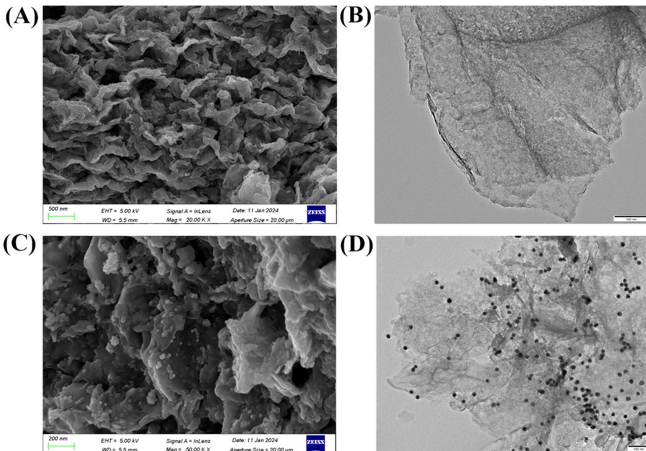
Fig. 1 SEM (A) and TEM (B) images of MoS<sub>2</sub> nanosheets. SEM (C) and TEM (D) images of MoS<sub>2</sub>@AuNP nanocomposites.
