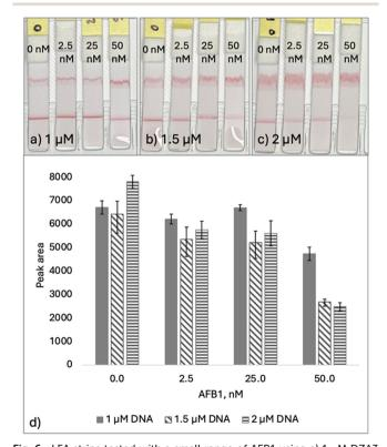
Fig. 6 LFA strips tested with a small range of AFB1 using a) 1  $\mu$ M DZA3 aptamer, b) 1.5  $\mu$ M DZA3 aptamer and c) 2  $\mu$ M DZA3 aptamer. d) Quantification of the signal change at the test zones using ImageJ.
