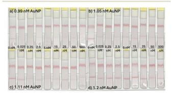
Fig. 7 Optimization of the concentration of AuNP to reduce the formation of DZA3-AFB1-AuNP complex to improve sensitivity. Image shows 1.5  $\mu$ M DZA3 with varying concentration of AFB1 an a) 0.99 nM AuNP, b) 1.05 nM AuNP, c) 1.11 nM AuNP and d) 1.20 nM AuNP.
