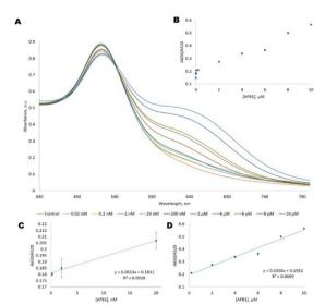
Fig. 5 A) Spectral changes to AuNP visible absorbance spectrum due to the aptamer's interaction with varying concentrations of AFB1 target ([0, 0.02, 0.2, 2, 20, 200 nM], [2, 4, 6, 8, 10  $\mu$ M]); B) ratio of the absorbance at 640 nm and 520 nm; C) and D) points of linearity used to determine the LOD, which were 2.28 nM and 1.81  $\mu$ M. Error bars represent standard error.
