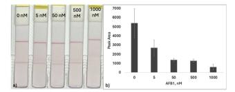
Fig. 10 Analysis of spiked peanut samples for the presence of AFB1. A) The AuNP-based LFA showing the decrease in test zone intensity as AFB1 concentration is increased. B) Histogram of peak area intensities calculated using ImageJ.
