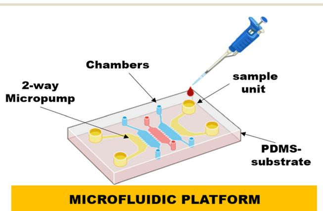
Fig. 7 Diagrammatic representation of dengue virus-based microfluidic platform.
