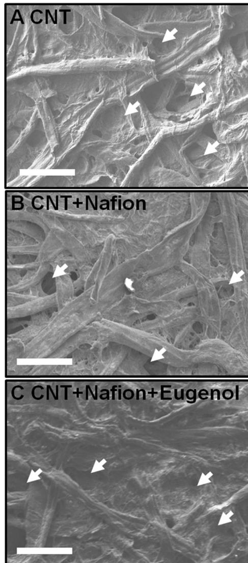
Fig. 3 Typical SEM images for different paper preparations: (A) paper/CNT, (B) paper/CNT/Nafion and (C) paper/CNT/Nafion/eugenol. Scale bars:  $100 \mu\text{m}$ . The arrows highlight the presence of large pores on all the micrographs.
