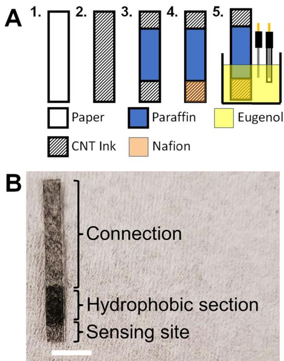
**Fig. 1** Fabrication of the NO sensors. (A) Schematic showing the preparation protocol: (1) cutting paper pieces, (2) coating in CNT ink, (3) blocking part of the paper with paraffin, (4) depositing Nafion and (5) electropolymerizing eugenol. (B) Photograph of the final device showing the different parts of the paper electrode (scale bar: 5 mm).
