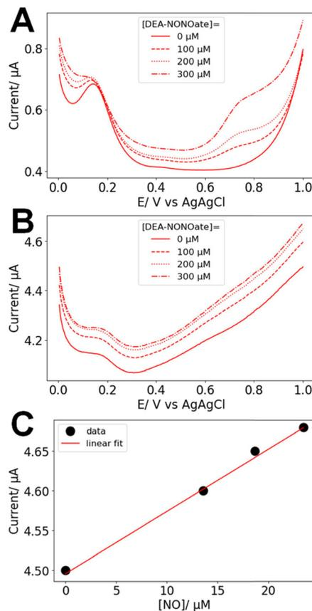
Fig. 6 Typical DPV recorded in PBS alone or supplemented with 100, 200, and 300  $\mu\text{M}$  DEA-NONOate for (A) glassy carbon and (B) a typical paper NO sensor. (C) DPV calibration curve for the data recorded from the typical NO sensor presented in (B).
