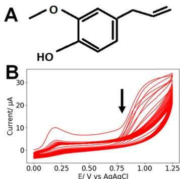
**Fig. 2** (A) Chemical structure of eugenol. (B) Typical CVs recorded during the electrodeposition of 0.1 mM eugenol in 0.1 M NaOH (25 cycles, SR = 100 mV s<sup>-1</sup>). The arrow indicates the order of the scans.
