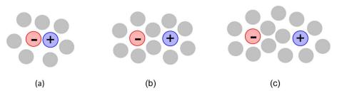
Fig. 1 (a) Contact IP (b) solvent-shared IP and (c) solvent-separated IP in molecular solvents.
