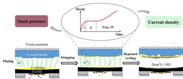
Unraveling plating/stripping-induced strain evolution *via* embedded sensors for predictive failure mitigation in solid-state Li metal batteries
