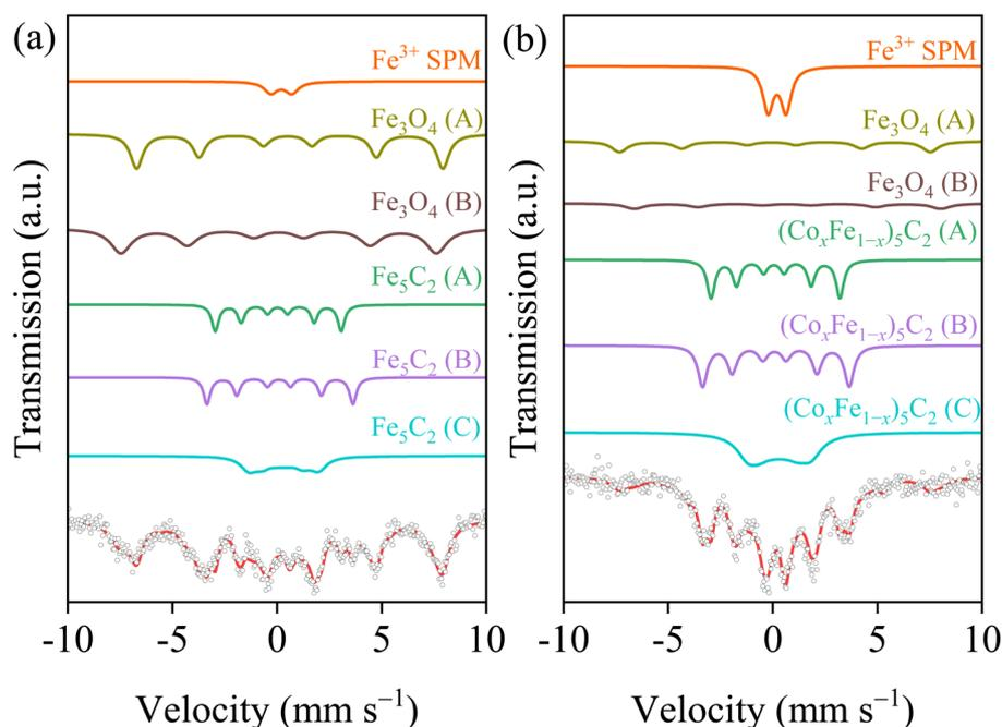
Fig. 6 <sup>57</sup>Fe Mössbauer spectra of the spent (a) Co<sub>0</sub>Fe and (b) Co<sub>1</sub>Fe<sub>2</sub> catalysts.
