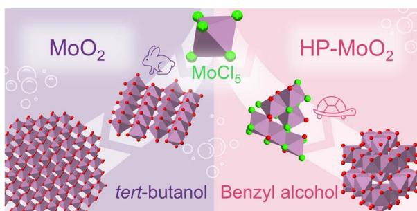
**Mechanistic insights into solvent-guided growth and structure of  $\text{MoO}_2$  nanoparticles in solvothermal synthesis**
