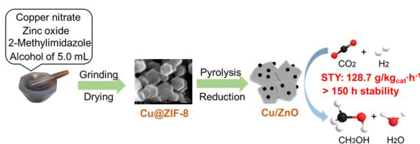
**Fast synthesis of Cu@zeolitic imidazolate framework-8 (ZIF-8) derived Cu/ZnO catalysts via a facile mechanical grinding method for CO<sub>2</sub> hydrogenation to methanol**
