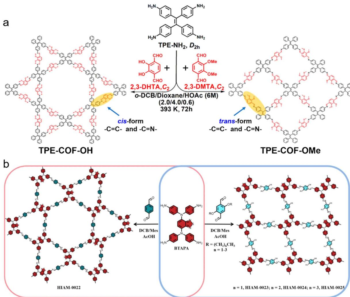
Fig. 11 (a) Topological structure modulation by side-chain chemistry.<sup>106</sup> Copyright 2020, American Chemical Society. (b) Conformational rearrangement through side-chain extension.<sup>109</sup> Copyright 2025, Royal Society of Chemistry.
