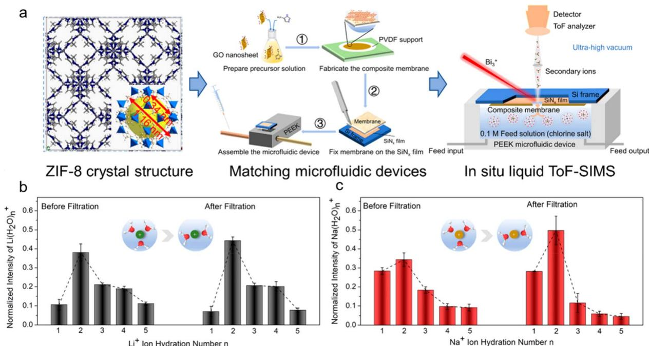
Fig. 2 Hydration structure characterization. (a) Schematic of the ZIF-8 structure and microfluidic technology coupled with *in situ* liquid ToF-SIMS analysis. The hydration structure of (b)  $\text{Li}^+$  and (c)  $\text{Na}^+$  before and after filtration.<sup>55</sup> Copyright 2023, American Chemical Society.
