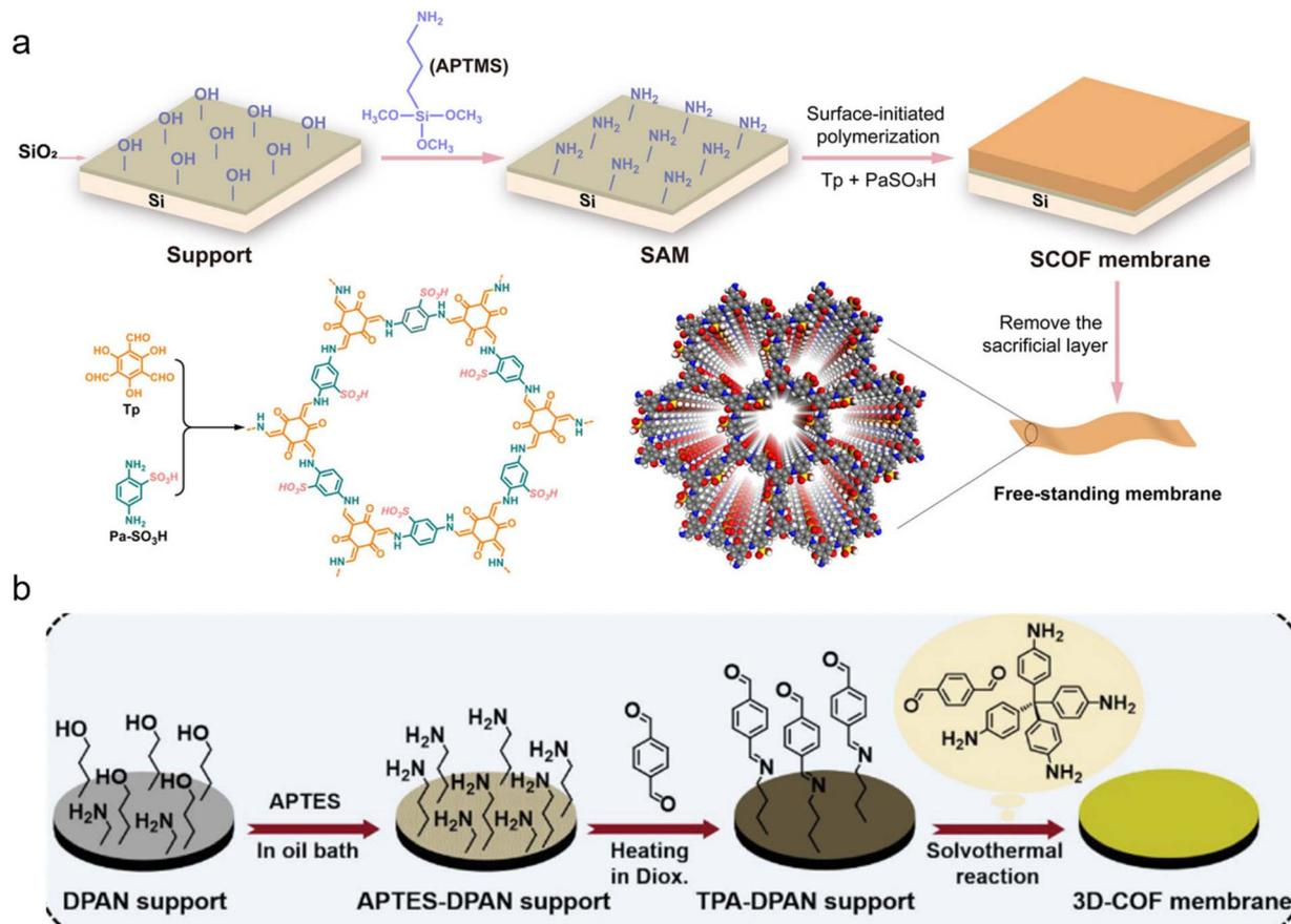
Fig. 14 (a) APTES monolayer initiated COF growth on silicon wafers.<sup>164</sup> Copyright 2021, Wiley-VCH. (b) Aldehyde-functionalized PAN substrates.<sup>169</sup> Copyright 2025, Wiley-VCH.
