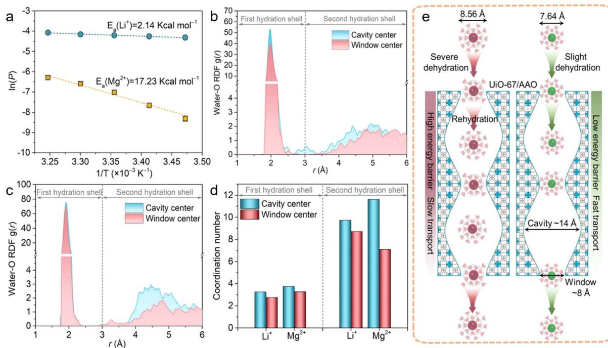
Fig. 3 Mechanistic insights into  $\text{Li}^+/\text{Mg}^{2+}$  separation. (a) Ionic conductivity experiments. RDFs for (b)  $\text{Li}^+$  and (c)  $\text{Mg}^{2+}$  positioned at both cavity and window centers of UiO-67. (d) First and second hydration shells of  $\text{Li}^+$  and  $\text{Mg}^{2+}$  at diverse channel positions. (e) Proposed mechanism for  $\text{Li}^+$  and  $\text{Mg}^{2+}$  transport.<sup>71</sup> Copyright 2021, Wiley-VCH.
