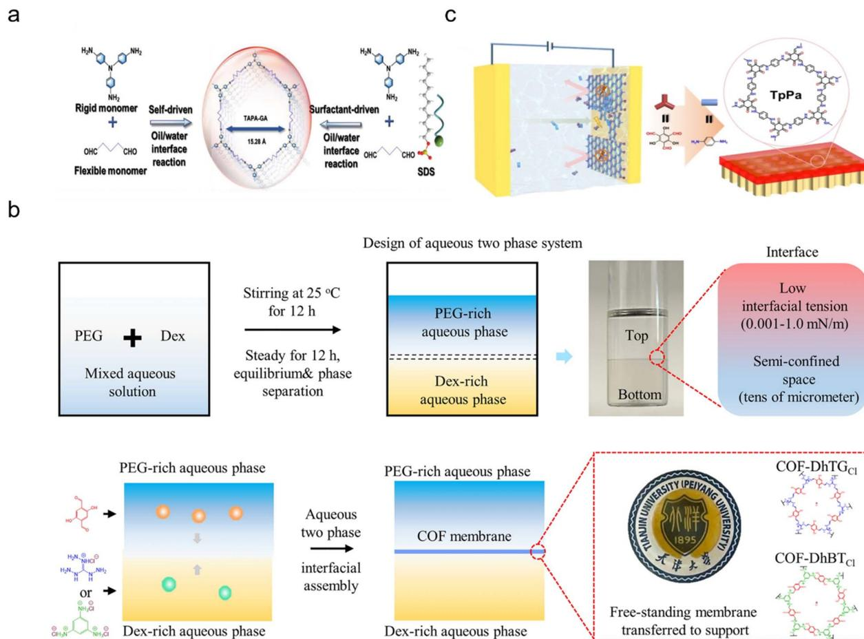
Fig. 16 (a) Surfactant-assisted interface polymerization.<sup>184</sup> Copyright 2023, Wiley-VCH. (b) Schematic of aqueous two-phase interface polymerization.<sup>187</sup> Copyright 2023, Wiley-VCH. (c) Electrochemical interface polymerization for ultrathin COF membrane fabrication.<sup>188</sup> Copyright 2022, Springer.
