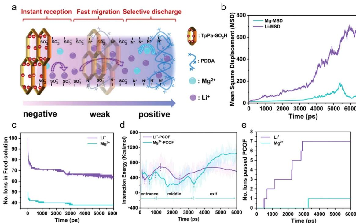
Fig. 7 Lithium–magnesium separation in heterocharged COF membranes. (a) Schematic of heterocharged nanochannels. (b) MSD of  $\text{Mg}^{2+}/\text{Li}^+$ . (c) Quantity of  $\text{Li}^+$  and  $\text{Mg}^{2+}$  in feed-solution. (d) Binding energy between ions and the COF. (e) Ion transport numbers across COFs.<sup>70</sup> Copyright 2024, Wiley-VCH.
