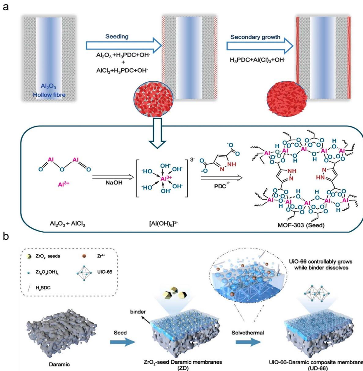
Fig. 17 (a) Bimetallic-source secondary growth strategy for MOF membrane fabrication.<sup>198</sup> Copyright 2024, Springer. (b) Seed-polymer blended to fabricate the substrate for MOF membrane synthesis.<sup>201</sup> Copyright 2021, Elsevier.
