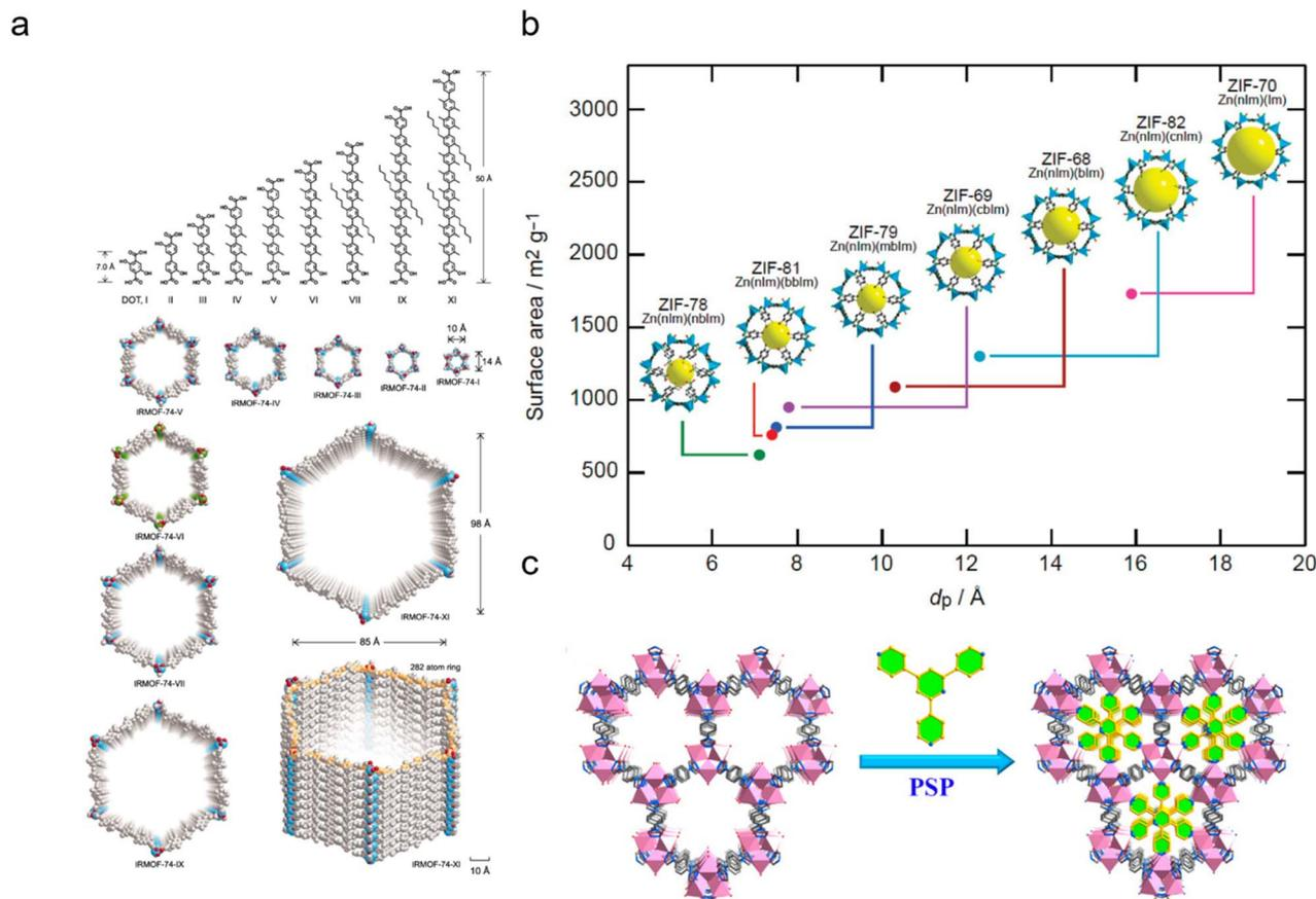
Fig. 13 (a) Engineering MOF architecture *via* design of organic ligands.<sup>140</sup> Copyright 2012, The American Association for the Advancement of Science. (b) Engineering MOF architecture *via* side chains.<sup>141</sup> Copyright 2009, American Chemical Society. (c) Pore space partitioning through axially coordinated organic units.<sup>144</sup> Copyright 2019, American Chemical Society.
