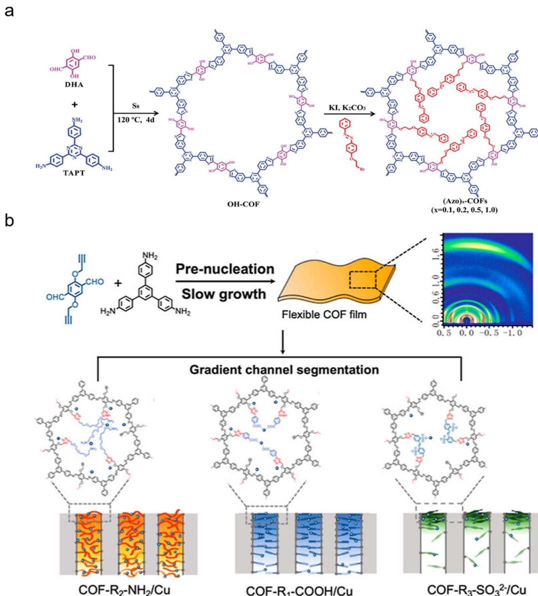
Fig. 12 (a) Incorporating stimuli-responsive units through post-synthetic modification.<sup>126</sup> Copyright 2024, Wiley-VCH. (b) Gradient channel segmentation *via* click reaction.<sup>136</sup> Copyright 2023, American Chemical Society.
