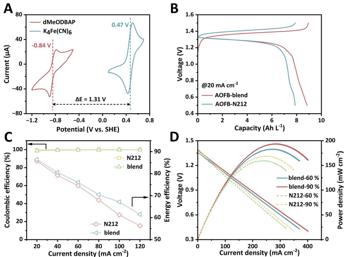
Fig. 2 The redox activity of dMeODABP. (A) CV curves of 5 mM dMeODABP and 10 mM K<sub>4</sub>Fe(CN)<sub>6</sub> dissolved in 1 M KOH solutions, respectively. (B) Charge and discharge curves of AOFB-blend and AOFB-N212 under 20 mA cm<sup>-2</sup>. (C) Coulombic efficiency and energy efficiency at different current densities for AOFB-blend and AOFB-N212. (D) Cell voltage and power density versus current density at different SOC for AOFB-blend and AOFB-N212.
