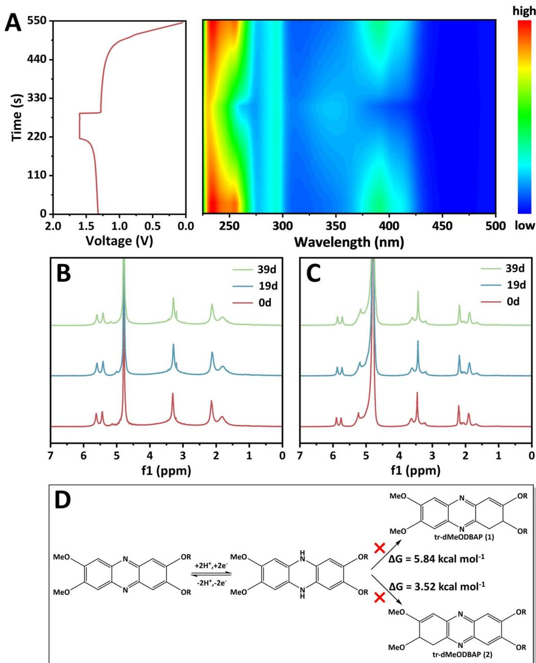
Fig. 3 Redox reversibility and chemical stability of dMeODBAP. (A) Voltage–time curve and corresponding 2D color filled contour plot of the *in situ* UV-vis test. (B) Time-dependent <sup>1</sup>H NMR spectroscopy data for 0.2 M dMeODBAP in 1 M KOH solution. (C) Time-dependent <sup>1</sup>H NMR spectroscopy data for 0.2 M re-dMeODBAP in 1 M KOH solution. (D) The investigation of potential tautomerization pathways of dMeODBAP by DFT calculations.
