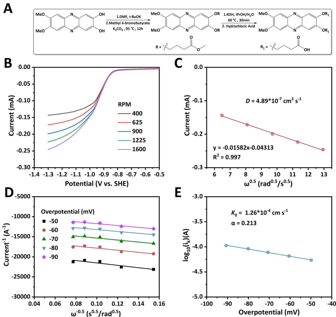
Fig. 1 Synthesis and redox kinetics study of dMeODBAP. (A) A scheme showing the synthesis route of dMeODBAP. (B) LSV curves at a scan rate of  $10 \text{ mV s}^{-1}$  at different rotation rates. (C) Levich plot of the limiting currents vs. the square roots of rotation rates. (D) Koutecky–Levich plots at different overpotentials, respectively. (E) Fitting plot of the Butler–Volmer equation at different overpotentials.
