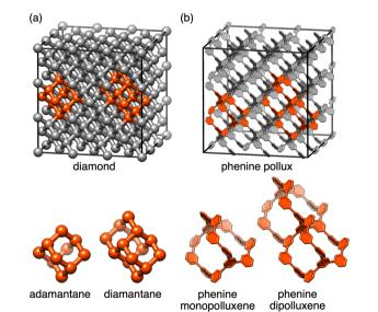
Fig. 1 Strongly isotropic nets of carbon atoms. (a) Diamond and its molecular segments (adamantane and diamantane). (b) Phenine pollux and its molecular segments (monopolluxene and dipolluxene).
