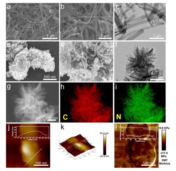
Fig. 2 Structural characterization studies of PZ-CHPT. SEM images of (a and b) PZ-CHPD and (d and e) PZ-CHPT. TEM images of (c) PZ-CHPD and (f) PZ-CHPT. (g-i) EDS analysis mapping images of PZ-CHPT. (j) AFM image, (k) 3D AFM image and (l) elastic modulus mapping of the top surface of PZ-CHPT.
