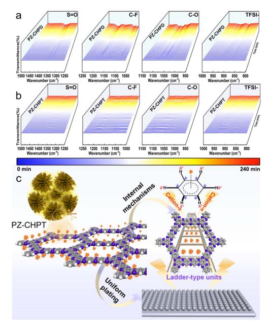
Fig. 6 In situ FT-IR analysis of electrolyte consumption in (a) PZ-CHPD and (b) PZ-CHPT modified Li symmetric cells. (c) The mechanism explanation of the PZ-CHPT film in enhancing Li<sup>+</sup> desolvation, migration, and the Li deposition process.
