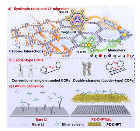
Fig. 1 Schematic illustration of the structural design and mechanism of PZ-CHPT. (a) Fabrication process and the Li<sup>+</sup> migration mechanism for the PZ-CHPT protective layer. (b) Double-stranded (ladder-type) COPs. (c) Morphology evolution during the deposition on bare Li and Li@PZ-CHPT.
