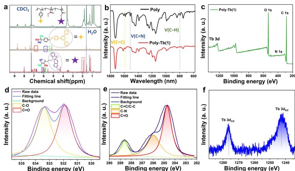
Fig. 2 Structural characterization of Poly and Poly-Tb(1): (a) comparison of <sup>1</sup>H NMR spectra of VTPY, SP and Poly; (b) FTIR spectra of Poly and Poly-Tb(1); (c) XPS survey spectrum of Poly-Tb(1); (d–f) high-resolution XPS spectra of C 1s, O 1s, and Tb 3d regions, respectively.
