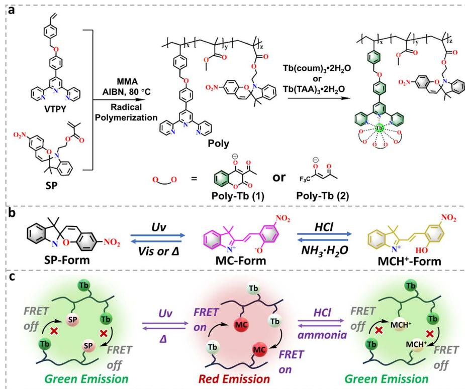
Fig. 1 (a) Synthetic procedures for Poly and Poly-Tb(1–2); (b) schematic illustration of the spiropyran moiety's response mechanisms to light, temperature, and acid/base stimuli; (c) multi-stimuli-responsive behavior of the lanthanide metallopolymer system.
