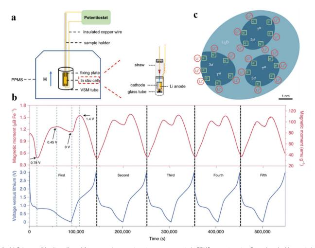
Fig. 5 (a) Scheme of in situ cell used for operando magnetometry measurements in PPMS magnetometer. Reproduced with permission.<sup>77</sup> Copyright 2022, American Chemical Society. (b) In situ magnetometry in an  $Fe_3O_4/Li$  cell as a function of electrochemical cycling under an applied magnetic field of 3 T. (c) Formation of a space charge zone in the surface capacitance model for extra lithium storage. Reproduced with permission.<sup>79</sup> Copyright 2021, Nature Publishing Group
