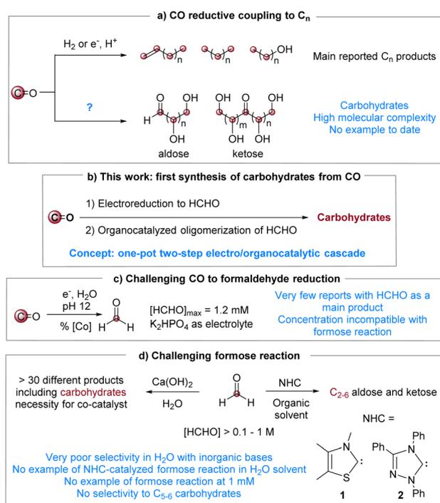
Scheme 1 (a) CO conversion to  $C_n$  compounds; (b) overview of the present work; (c) status and challenges of CO to HCHO electro-conversion; (d) status and challenges of formose reaction catalyzed by inorganic base (in  $\text{H}_2\text{O}$ ) and by NHC (in organic solvent).
