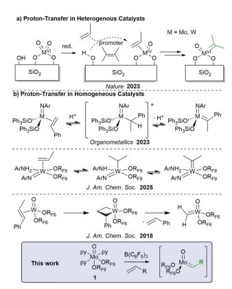
Fig. 1 Formation of alkylidene active species in (a) heterogeneous and (b) homogeneous catalytic systems.  $OR_{F6} = OC(CF_3)_2CH_3$ ,  $OR_{F9} = OC(CF_3)_3$ .
