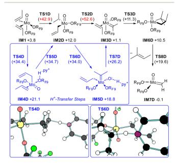
Fig. 6 Activation through allyl-alkyl mechanism: minimum-energy reaction pathway, calculated at the B3LYP-D3(BJ)/def2-TZVP level of theory. Gibbs free energies in kcal mol<sup>-1</sup> relative to intermediate IM0.
