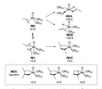
Fig. 4 Computed Gibbs free energies ( $\Delta G$ , kcal mol<sup>-1</sup>) of the first intermediates generated through vinylic and allylic C-H activation, or oxidative coupling yielding metallacyclopentanes. Calculated at the B3LYP-D3(BJ)/def2-TZVP level of theory. Gibbs free energies in kcal  $mol^{-1}$  relative to intermediate IM0.
