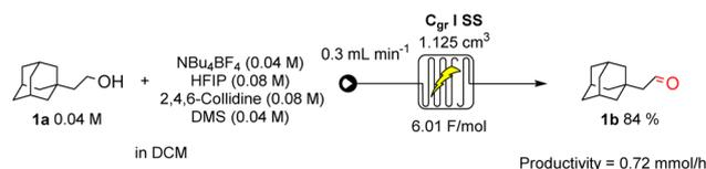
Scheme 4 Optimised continuous flow conditions for the eCarbonyls reaction.
