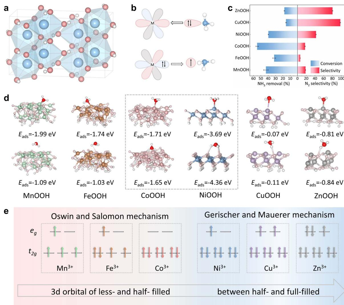
Fig. 1 (a) Crystal structure of MOOH; (b) different adsorption types with  $\text{NH}_3$ ; (c) EAOR activity and selectivity of MOOH with different transition metal ions ( $E = 1.8 \text{ V}$ ,  $\text{pH} = 11$ ,  $0.05 \text{ M Na}_2\text{SO}_4$ ); (d) calculated adsorption energies of ammonia molecules at metal and hydroxyl sites in mono-metallic oxyhydroxides; (e) diagram of d orbital electron configuration of different transition metal ions.
