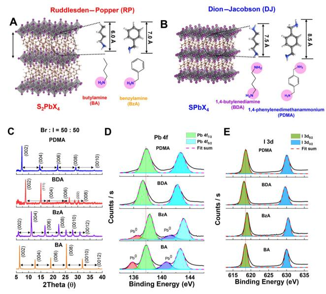
Fig. 1 (A and B) Crystal structures of 2D RP perovskites with a formula of  $S_2PbX_4$  (A) and 2D DJ perovskites with a formula of  $SPbX_4$  (B). (C) XRD patterns obtained for 2D mixed halide perovskites of Br : I = 50 : 50 with BA, BzA, BDA, and PDMA as spacers. (D and E) XPS spectra for Pb 4f and I 3d recorded for 2D mixed halide perovskites with BA, BzA, BDA, and PDMA as spacers from bottom to top.
