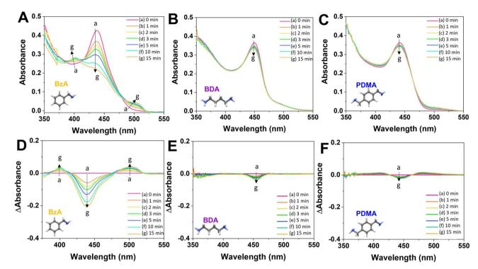
Fig. 4 (A–C) Time-dependent absorption changes and (D–F) corresponding difference absorption changes for 15 minutes recorded for 2D mixed halide perovskites with (A and D) BzA, (B and E) BDA, and (C and F) PDMA, respectively, upon CW 405 nm laser irradiation (100 mW cm $^{-2}$ ) for 15 minutes. In the difference absorption spectra, the 0 min spectrum serves as a reference spectrum for subtraction.
