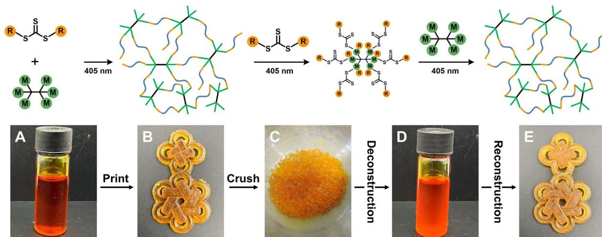
Fig. 3 Recyclable 3D printing. (A) The initial resin; (B) the printed Chinese knot; (C) the crushed Chinese knot; (D) the recycled resin; (E) the reprinted Chinese knot.
