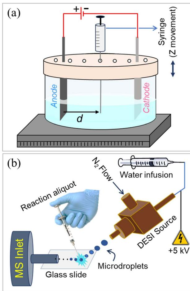
Fig. 1 (a) Diagram of the electrochemical reaction chamber with pre-defined sampling ports (holes) on the lid, strategically located at different distances from the anode ( $d$ ) to facilitate spatial sampling during the reaction. (b) A 10  $\mu\text{L}$  reaction aliquot withdrawn from the electrolytic cell was subjected to bombardment with positively charged water microdroplets in a DESI-MS setup, enabling rapid interception and detection of the reactive carbocation intermediate.
