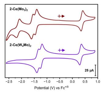
Fig. 4 Cyclic voltammograms of  $2\text{-Ce}(Mo_5)_2$  (maroon) and  $2\text{-Ce}(W_4Mo)_2$  (purple). The data was acquired in MeCN with 0.1 M TBA(PF<sub>6</sub>) supporting electrolyte, 1 mM of cluster, and a scan rate of 200 mV s<sup>-1</sup>.
