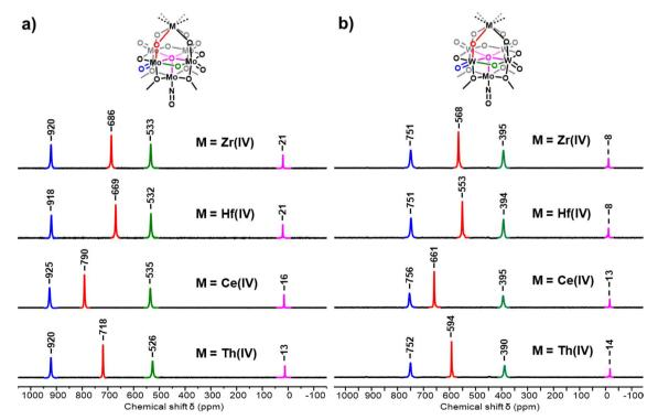
Fig. 8  $^{17}$ O NMR spectrum of (a) **3-Ce(Mo<sub>5</sub>)<sub>2</sub>** and (b) **3-Ce(W<sub>4</sub>Mo)<sub>2</sub>** compared to other isostructural M<sup>IV</sup> centered sandwich-type complexes. All spectra were obtained in CD<sub>2</sub>Cl<sub>2</sub> at room temperature.
