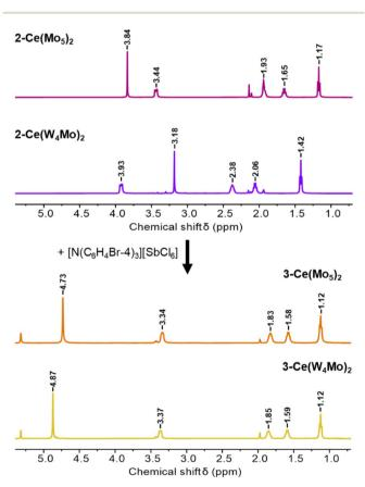
Fig. 6 <sup>1</sup>H NMR spectra following the one electron oxidation of 2- $Ce(Mo_5)_2$  and  $2-Ce(W_4Mo)_2$  by tris(4-bromophenyl)ammoniumyl hexachloroantimonate to give the Ce<sup>IV</sup> centered complexes 3- $Ce(Mo_5)_2$  and  $3-Ce(W_4Mo)_2$ . Spectra of the  $Ce^{\text{\tiny III}}$  complexes were obtained in  $CD_3CN$ , while the  $Ce^{iv}$  complexes were obtained in  $CD_2Cl_2$ . All spectra were recorded at room temperature.
