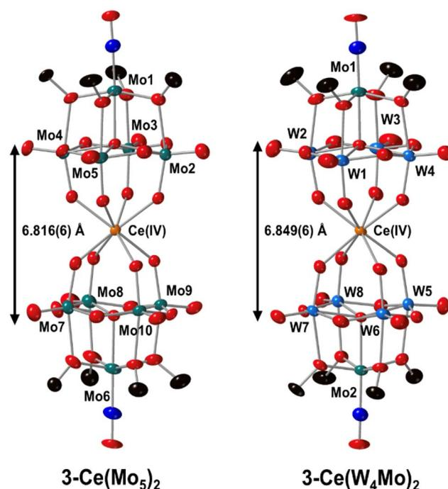
Fig. 7 SCXRD structures of the  $\text{Ce}^{\text{IV}}$  centered complexes  $3\text{-Ce}(\text{Mo}_5)_2$  and  $3\text{-Ce}(\text{W}_4\text{Mo})_2$  with probability ellipsoids set at 50%. The tetra-butylammonium cations, solvent molecules, and some disorder has been masked for clarity.
