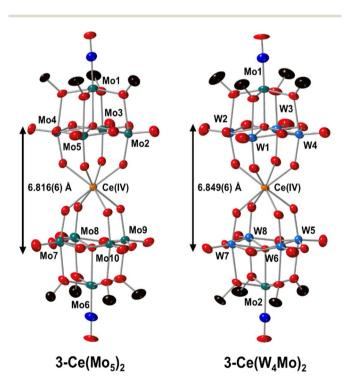
Fig. 7 SCXRD structures of the Ce<sup>IV</sup> centered complexes 3-Ce(Mo<sub>5</sub>)<sub>2</sub> and  $3-Ce(W_4Mo)_2$  with probability ellipsoids set at 50%. The tetrabutylammonium cations, solvent molecules, and some disorder has been masked for clarity.
