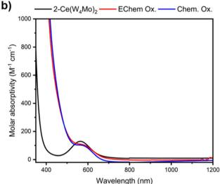
Fig. 5 UV-vis spectra of pristine  $2\text{-Ce}(Mo_5)_2$  (a, black) and  $2\text{-Ce}(W4Mo)_2$  (b, black) compared to those obtained after electrochemical oxidation (red) or chemical oxidation by tris(4-bromophenyl) ammoniumyl hexachloroantimonate (blue). All spectra were recorded in MeCN at room temperature.
