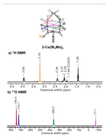
Fig. 2  $^{1}$ H NMR spectrum (a) and  $^{17}$ O NMR spectrum (b) of 2-Ce( $W_{4}$ Mo)<sub>2</sub>. Spectra were obtained in CD<sub>3</sub>CN at room temperature.
