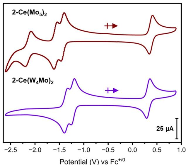
Fig. 4 Cyclic voltammograms of  $2\text{-Ce}(\text{Mo}_5)_2$  (maroon) and  $2\text{-Ce}(\text{W}_4\text{Mo})_2$  (purple). The data was acquired in MeCN with 0.1 M TBA(PF<sub>6</sub>) supporting electrolyte, 1 mM of cluster, and a scan rate of  $200 \text{ mV s}^{-1}$ .
