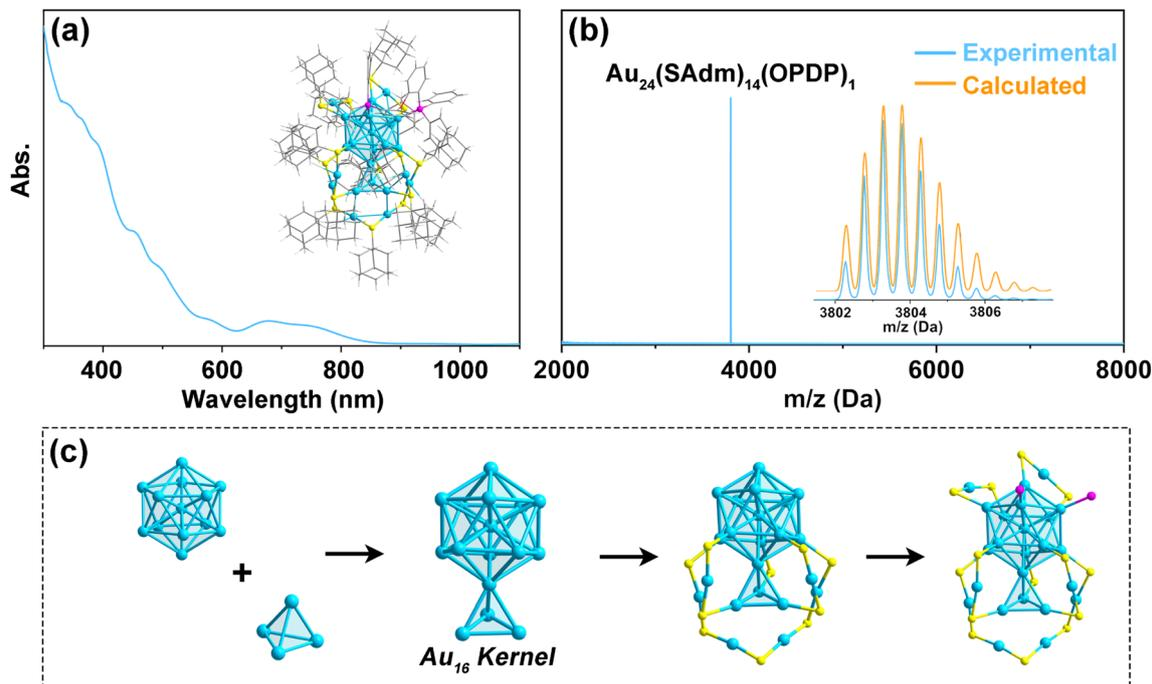
Fig. 1 (a) UV-vis spectrum of  $\text{Au}_{24}$ . Inset: total structure of  $\text{Au}_{24}$ . (b) ESI-MS of  $\text{Au}_{24}$ . Inset: experimental and calculated isotopic patterns of the MS signal. (c) Structural analysis of the skeleton in  $\text{Au}_{24}$ . (Labels: light blue = Au; yellow = S; magenta = P; gray = C; red = O; white = H).
