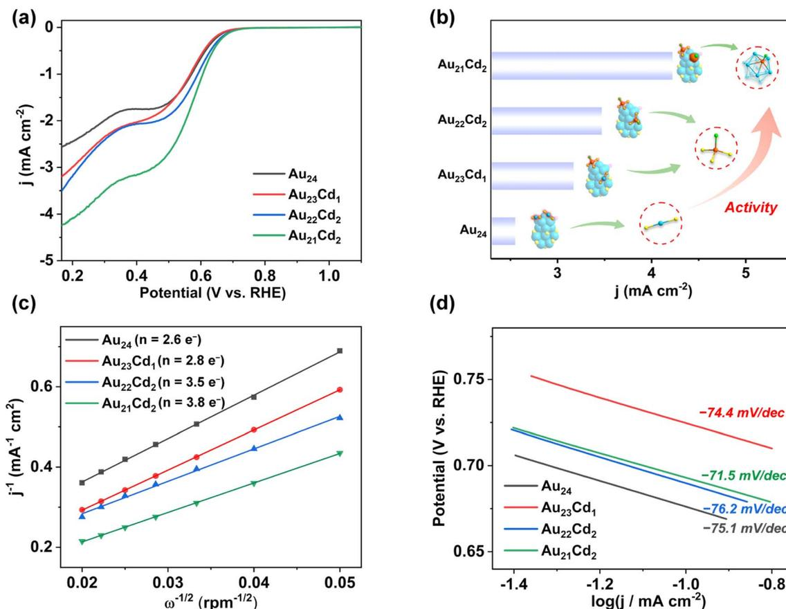
Fig. 4 (a) ORR polarization curves for different NCs as catalysts obtained in O<sub>2</sub>-saturated 0.1 mol per L KOH solutions at 1600 rpm. (b) The current density values for different NCs as catalysts (0.17 V, 1600 rpm) and the corresponding different local structures of these NCs. (c) Koutecky–Levich plots ( $j^{-1}$  vs.  $\omega^{-1/2}$ ) of different NCs. (d) Corresponding Tafel plots of the NCs.
