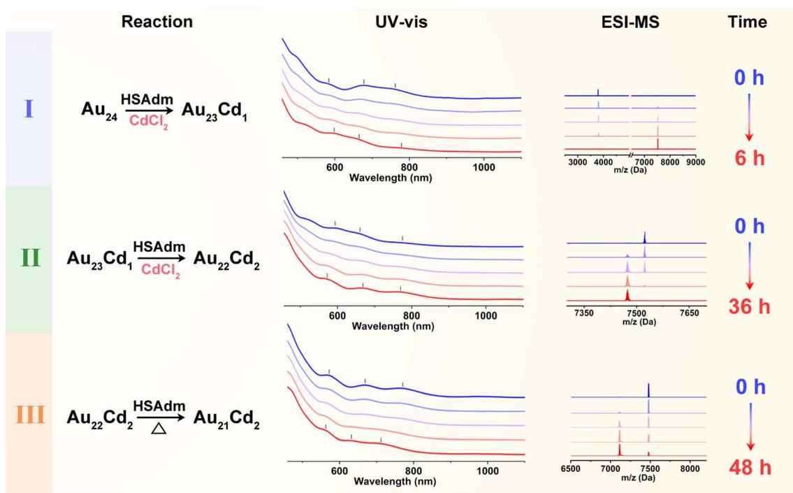
Fig. 2 Reaction system composition and the time-dependent UV-vis spectra and ESI-MS of the three transformation stages, including  $\text{Au}_{24}$  to  $\text{Au}_{23}\text{Cd}_1$  (stage I),  $\text{Au}_{23}\text{Cd}_1$  to  $\text{Au}_{22}\text{Cd}_2$  (stage II), and  $\text{Au}_{22}\text{Cd}_2$  to  $\text{Au}_{21}\text{Cd}_2$  (stage III).
