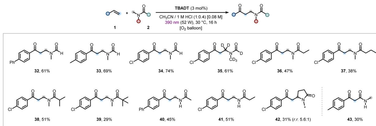
Fig. 3 Scope of the alkene oxo-amidomethylation varying amide partner. Reaction conditions: styrene **1** (0.3 mmol, 1.0 equiv.), amide **2** (1.5 mL), **TBADT** (3 mol%), 1 M aqueous HCl (0.6 mL) in anhydrous CH<sub>3</sub>CN (1.5 mL). For further details, see the SI. Isolated yields are reported.
