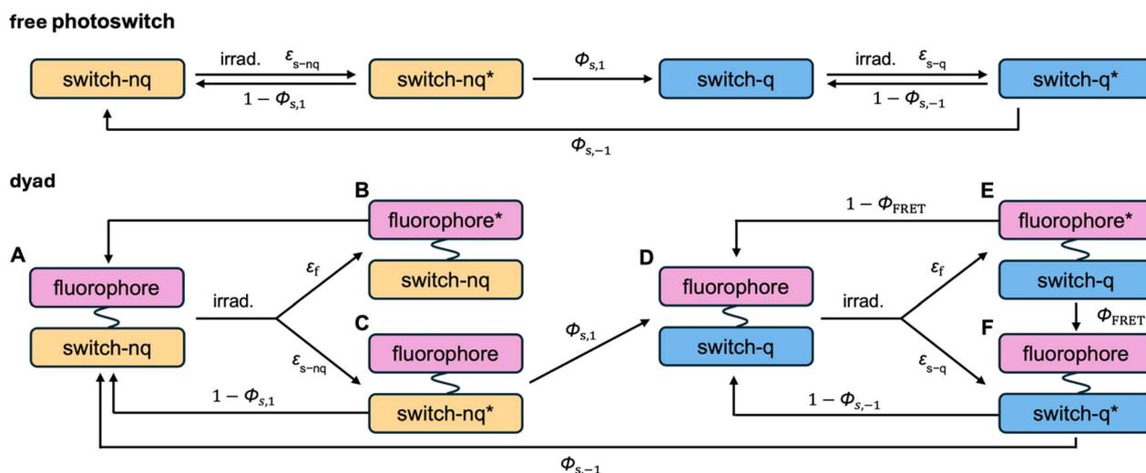
**Fig. 5** Schematic photophysical model showing the possible states that can be accessed by a photoswitch (top) and a photoswitch-fluorophore dyad (bottom). (A–F) denote different energetic states.
