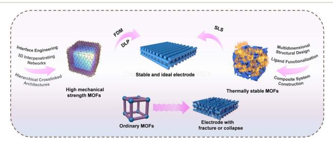
Fig. 5 Enhancing MOF-based electrode performance: the critical role of high mechanical strength MOFs, thermally stable MOFs, and multi-dimensional structural design in electrode fabrication *via* advanced 3D printing techniques.
