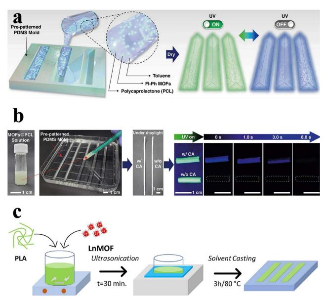
Fig. 12 (a) Diagram illustrating the fabrication process of PCL filaments embedded with FI MOF and FI-Ph MOF particles, produced using a prepatterned PDMS mold. (b) Images capturing the stepwise fabrication of Fl-Ph MOF@PCL filaments, demonstrating the retention of dual luminescent properties throughout the process. (c) Diagram illustrating the processing workflow for PLA/LnMOF composite materials.
