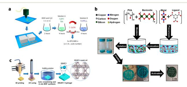
Fig. 14 (a) Preparation of composite materials integrating Cu-BTC with ABS. (b) Stepwise fabrication mechanism of HKUST-1 monoliths through the novel GPG strategy. (c) Visual protocol for the 3D bioprinting cascade: sequential deposition, UV-triggered solidification, and electrolytemediated crosslinking.
