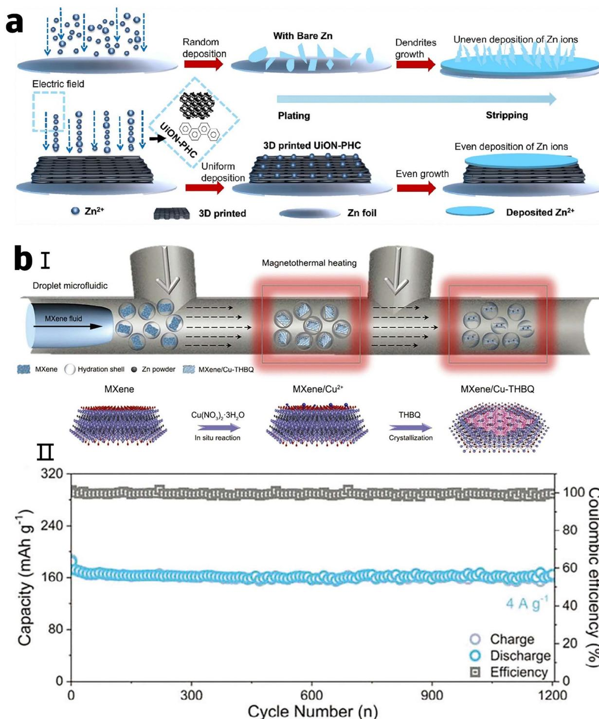
**Fig. 18** (a) Schematic illustration of Zn<sup>2+</sup> deposition mechanisms on bare Zn versus 3D-printed UiON-PHC composite anodes. (b) (I) Microfluidic synthesis of MXene/Cu-THBQ/Zn-P printable hybrid ink and heterostructured composite formation mechanism. (II) Long-term cycling performance (4 A g<sup>-1</sup>) of M3DP-MXene/Cu-THBQ/Zn-P//G-TEMPO full battery, demonstrating high-rate stability and extended lifespan.
