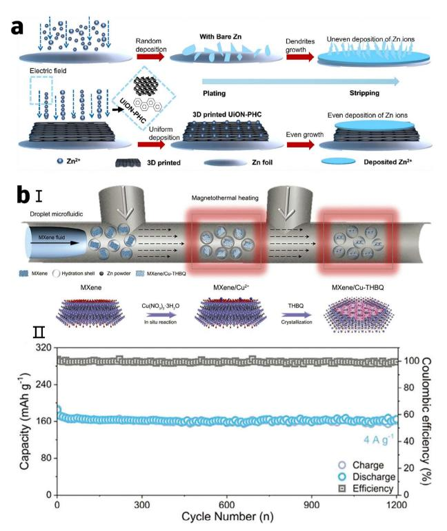
Fig. 18 (a) Schematic illustration of Zn2+ deposition mechanisms on bare Zn versus 3D-printed UiON-PHC composite anodes. (b) (I) Microfluidic synthesis of MXene/Cu-THBQ/Zn-P printable hybrid ink and heterostructured composite formation mechanism. (II) Long-term cycling performance (4 A g-1) of M3DP-MXene/Cu-THBQ/Zn-P//G-TEMPO full battery, demonstrating high-rate stability and extended lifespan.
