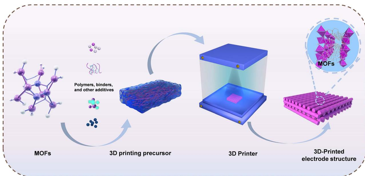
Fig. 1 The strategy for preparing mof into 3D printing precursors and the 3D printing schematic diagram.
