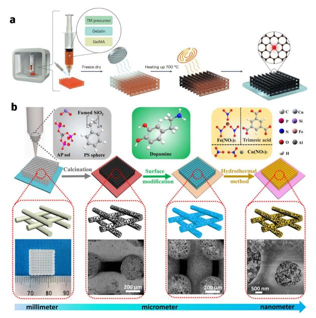
Fig. 15 (a) Layer-by-layer assembly methodology for SAC composites in 3D printing. (b) Multistep architecture design: DIW-processed porous ceramics integrated with spatially ordered metal—organic frameworks.
