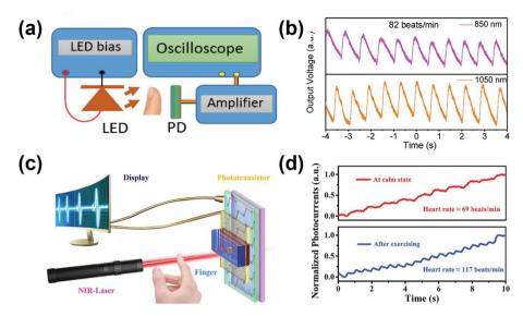
Fig. 13 (a) PPG measurement setup, (b) heartbeat waveforms measured under 850 nm and 1050 nm illumination of DPP-DTT:SWIR dye-based OPD PPG sensor. Reproduced from ref. 80 with permission from Wiley-VCH, copyright 2020. (c) NIR contactless real-time pulse monitoring setup, (d) heart rate of a subject at rest and post-exercise of PTB7-Th:IEICO-4F:PC<sub>71</sub>BM-based OPD PPG sensor. Reproduced from ref. 81 with permission from Wiley-VCH, copyright 2021.
