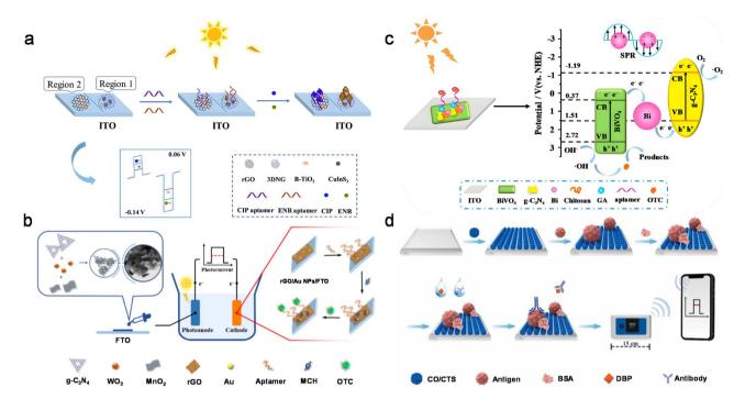
(a) Fabrication of the PEC aptasensor for detecting two antibiotics.<sup>94</sup> Copyright 2021, Elsevier. (b) Preparation of the sensor platform.<sup>95</sup> Copyright 2021, American Chemical Society. (c) Schematic illustration of the PEC aptasensor for OTC detection based on the Bi/BiVO<sub>4</sub>/q-C<sub>3</sub>N<sub>4</sub> heterojunction.96 Copyright 2020, Elsevier. (d) Construction process of the PEC POCT platform for detecting DBP.97 Copyright 2023, Elsevier.
