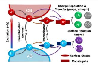
Fig. 2 A schematic depiction of the photocatalytic processes occurring across timescales from femtoseconds to seconds.<sup>40</sup> Copyright 2022, John Wiley and Sons.
