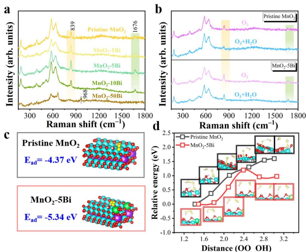
Fig. 3 *In situ* Raman spectra and DFT calculation results. (a) *In situ* Raman spectra of pristine  $\text{MnO}_2$  and  $\text{MnO}_2\text{-xBi}$  in ozone gas. (b) *In situ* Raman spectra of pristine  $\text{MnO}_2$  and  $\text{MnO}_2\text{-5Bi}$  with the addition of water. (c) Theoretical models of  $^{\circ}\text{OOOH}$  on  $\text{MnO}_2$  and  $\text{MnO}_2\text{-5Bi}$  catalysts. (d) Potential energy surface scanning for  $^{\circ}\text{OOOH}$  along the middle O-O bond.
