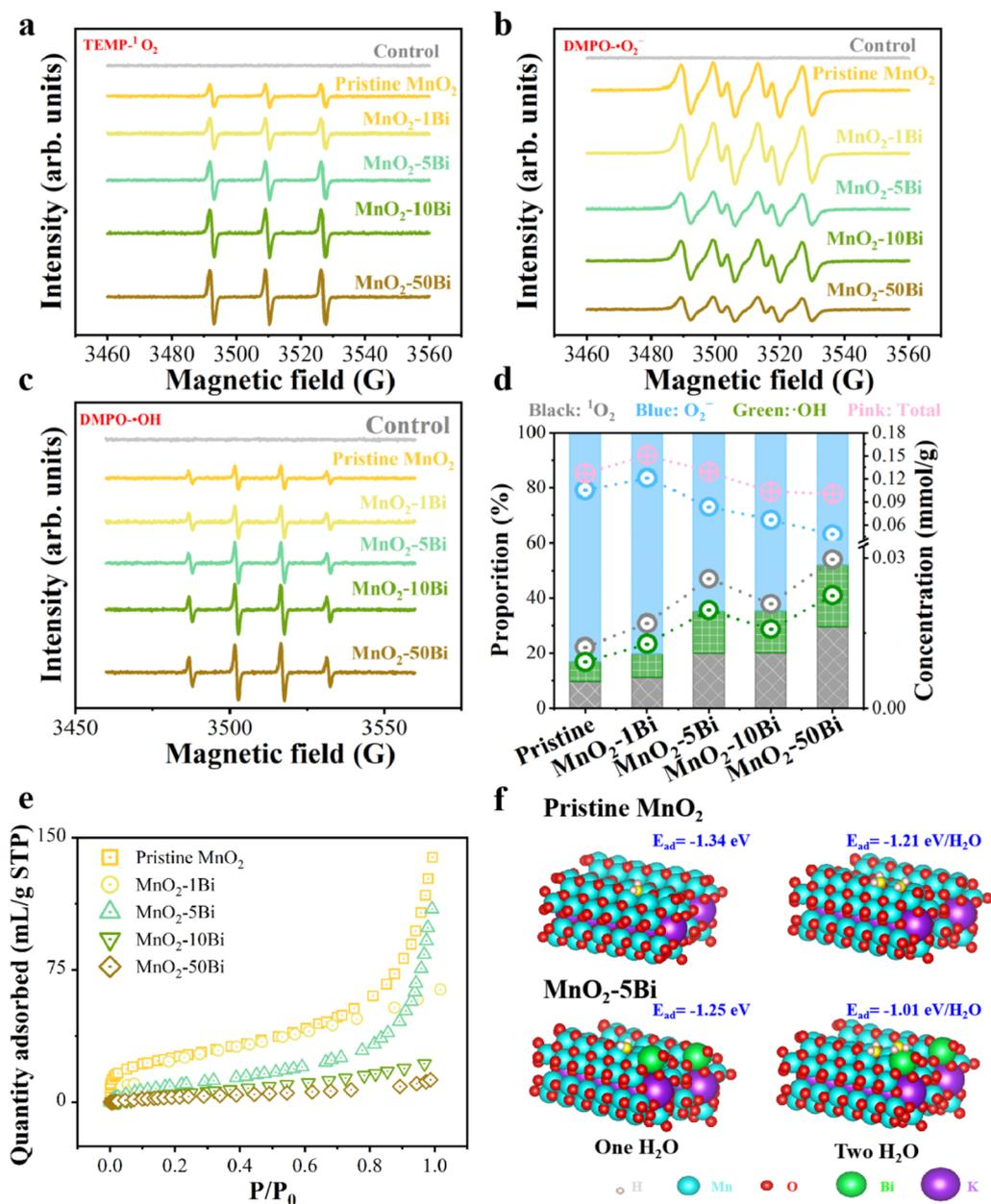
Fig. 2 Chemical properties of the pristine MnO<sub>2</sub> and MnO<sub>2</sub>-xBi catalysts. (a–d) ESR spectra of the ROS when the pristine MnO<sub>2</sub> and MnO<sub>2</sub>-xBi catalysts are exposed to O<sub>3</sub> in the dark. (e) Static adsorption isotherms for water. (f) Optimized adsorption structures for water on pristine MnO<sub>2</sub> and MnO<sub>2</sub>-Bi with dimer vacancies.
