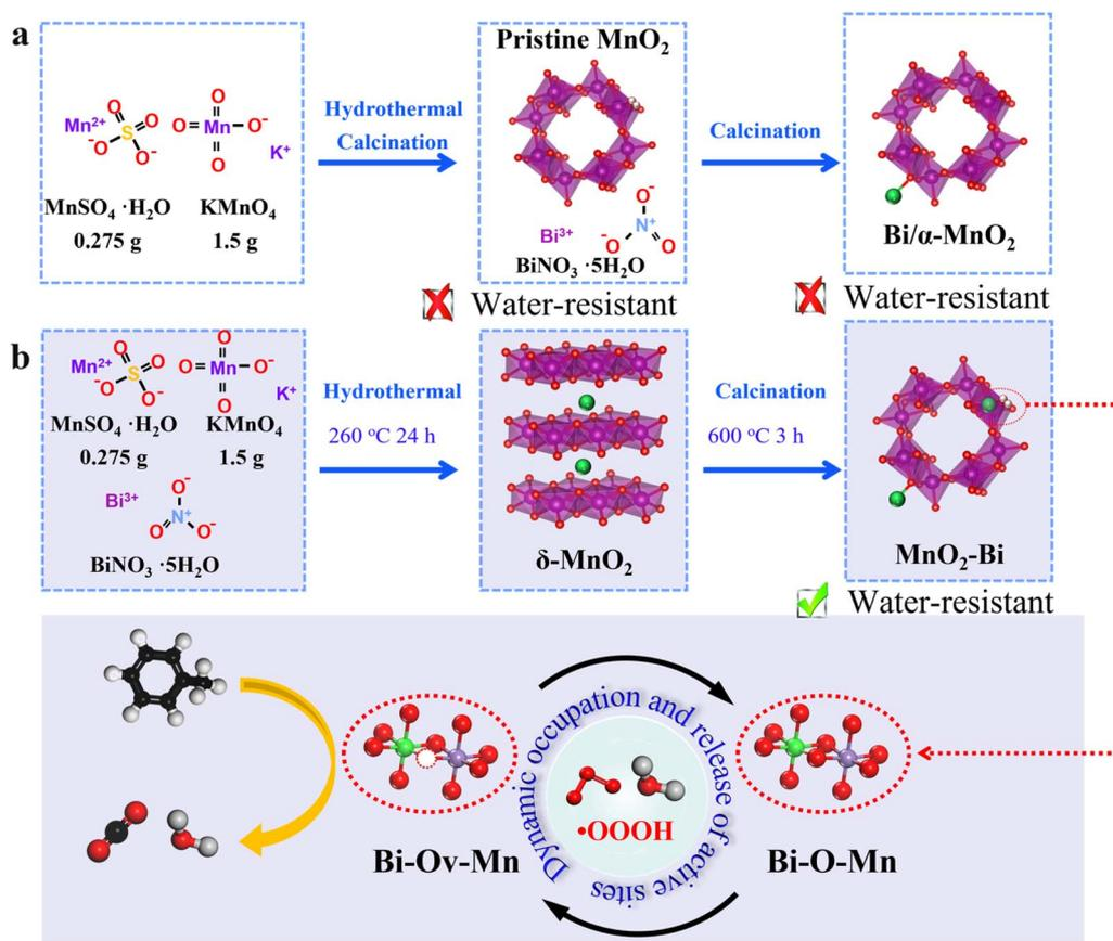
Scheme 1 Schematic diagram of catalyst preparation: (a) Bi/ $\alpha$ -MnO<sub>2</sub> and (b) MnO<sub>2</sub>-Bi.
