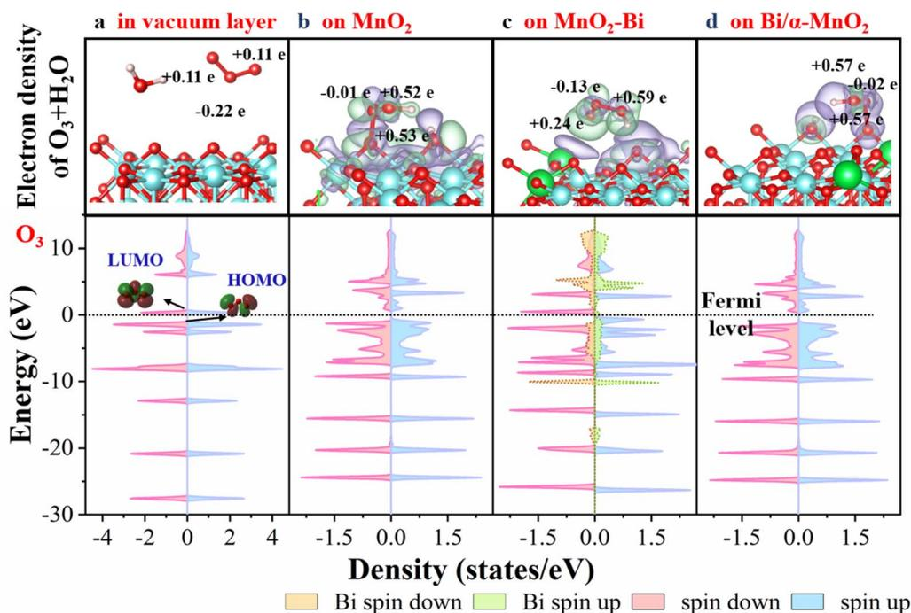
Fig. 4 Electron density difference and DOS analysis of O<sub>3</sub> for O<sub>3</sub> + H<sub>2</sub>O in the vacuum layer (a), on MnO<sub>2</sub> (b), on MnO<sub>2</sub>–Bi (c), and on Bi/α-MnO<sub>2</sub> (d). The cyan and green colours indicate a decrease and increase in the electron density, respectively.
