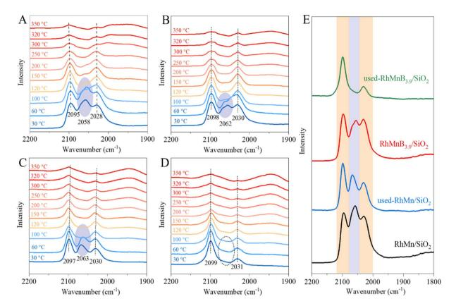
Fig. 3 CO-desorption in situ IR spectra of (A) RhMn/SiO<sub>2</sub>, (B) RhMnB<sub>3.9</sub>/SiO<sub>2</sub>, (C) used-RhMn/SiO<sub>2</sub> and (D) used-RhMnB<sub>3.9</sub>/SiO<sub>2</sub> catalysts at different temperatures. (E) CO-desorption in situ IR spectra at 30 °C. The data is collected from (A-D).
