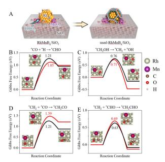
Fig. 4 (A) Models showing the optimization of the RhMnB<sub>x</sub>/SiO<sub>2</sub> catalyst structure during the reaction by spontaneous deposition of boron oxide species. (B-E) Gibbs free energy diagrams and configurations for four intermediate steps on  $Mn_1O_1$  supported on the Rh (111) facet (black line) and (221) facet (red line) at 595 K. The insets in (B-E) show the configurations of the initial state (IS), transition state (TS) and final state (FS) on Rh (111).
