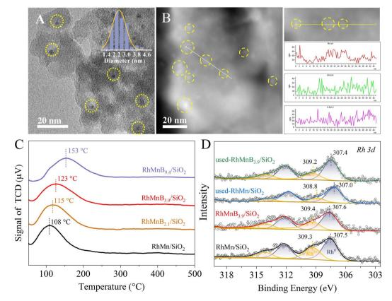
Fig. 2 (A) TEM image of the used-RhMnB $_{3.9}$ /SiO $_2$  after reaction for 118 h. The inset in (A) shows the metal nanoparticle size distribution. (B) STEM image and linear-scan EDS spectra of the used-RhMnB $_{3.9}$ /SiO $_2$  catalyst. The yellow circles highlight the nanoparticles. (C) H $_2$ -TPR profiles of various catalysts. (D) Rh 3d XPS spectra of reduced and used RhMn/SiO $_2$  and RhMnB $_3$ 9/SiO $_2$  catalysts.
