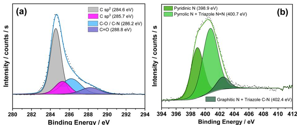
Fig. 2 (a) C 1s and (b) N 1s core level XPS regions of NG-C<sub>60</sub> (5) and their relative fits.
