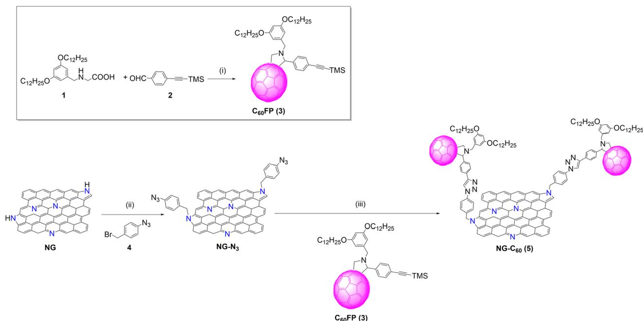
**Scheme 1** Synthetic route for the preparation of **NG-C<sub>60</sub>** (**5**) hybrid. Reagents and conditions: (i) C<sub>60</sub>, toluene, 6 h, reflux, 45%; (ii) K<sub>2</sub>CO<sub>3</sub>, NMP, 70 °C, 48 h, (iii) TBAF, THF, NMP, rt or 0 °C, 3 h; then, CuSO<sub>4</sub>·5H<sub>2</sub>O, sodium ascorbate, NMP, 70 °C, 48 h.
