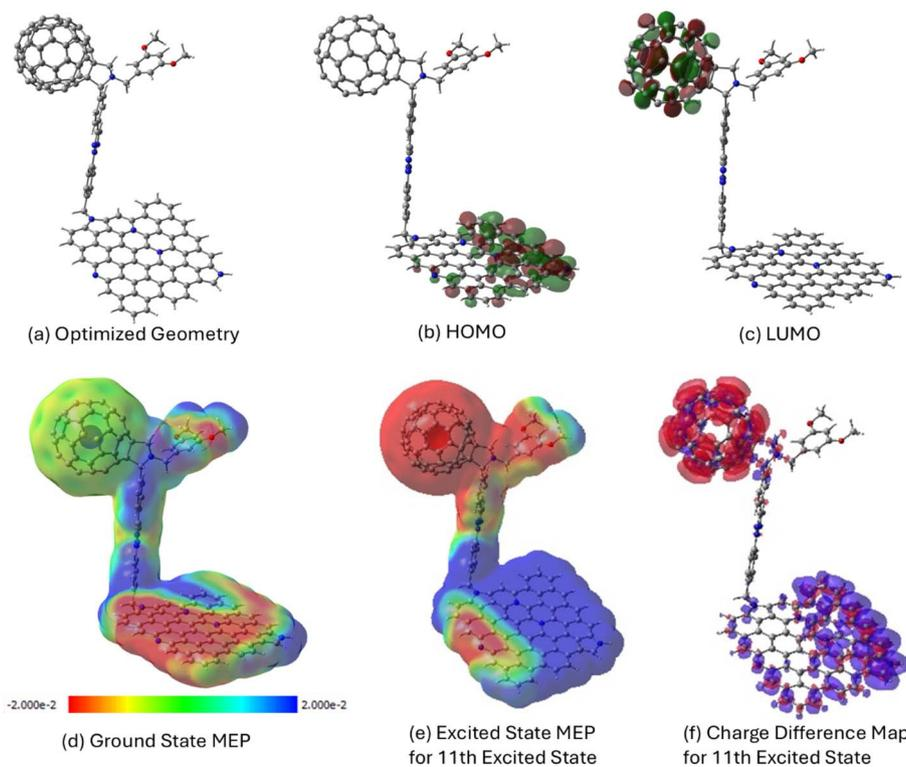
Fig. 4 (a) Optimized geometry, (b) HOMO, (c) LUMO, (d) ground state MEP, (e) first excited state MEP, and (f) charge difference map for the first excited state of NG-C<sub>60</sub> hybrid calculated at the CAM-B3LYP/6-311G(d,p) level with the SCRF-PCM solvation model in *o*-dichlorobenzene.
