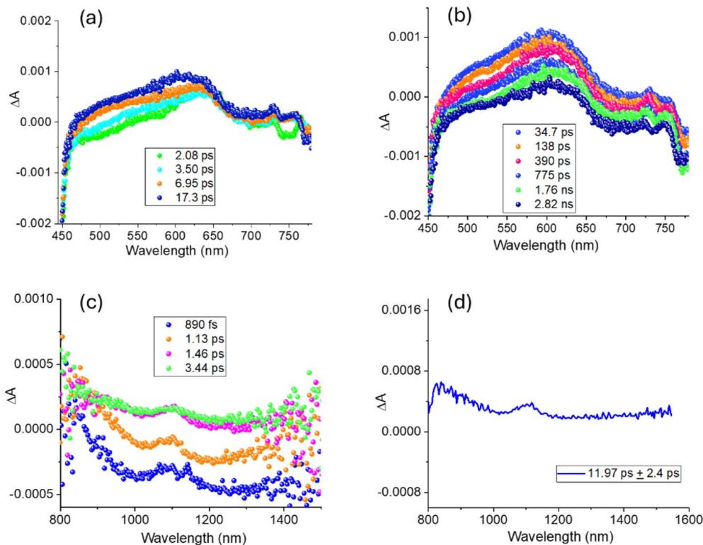
**Fig. 6** fs-TA spectra at the indicated delay times of the NG-C<sub>60</sub> hybrid (a and b covering the visible region and c covering the near-IR region). The result of global target analysis is shown in Fig. 6d. The sample was excited using a 100-fs pulsed laser tuned to 433 nm, corresponding to C<sub>60</sub> in DMF.
