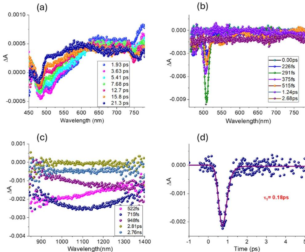
Fig. 5 fs-TA spectra at the indicated delay times of C<sub>60</sub> used in the click reaction, (b and c) of NG covering the visible and near-IR region, and (d) the NG exciton time profile. The samples were excited using a 100-fs pulsed laser tuned to 433 nm for C<sub>60</sub> and 440 nm for NG in DMF.
