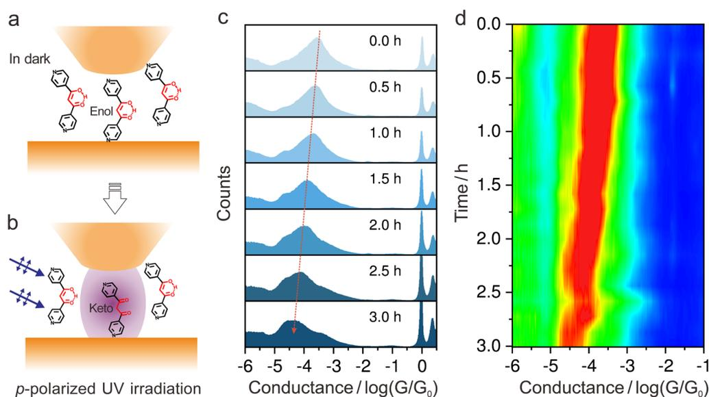
Fig. 3 Conductance evolution of BPPD-enol molecular junctions upon *in situ* UV irradiation in TCB. (a) Schematic diagram of the STM-BJ technique performed in dark in which BPPD exists in the enol form, and (b) under p-polarized laser irradiation in which BPPD-enol inside the nanogap was transformed to BPPD-keto. (c) 1D conductance histograms of BPPD-enol junctions during *in situ* UV irradiation. (d) 2D conductance evolution of BPPD-enol junctions upon UV irradiation.
