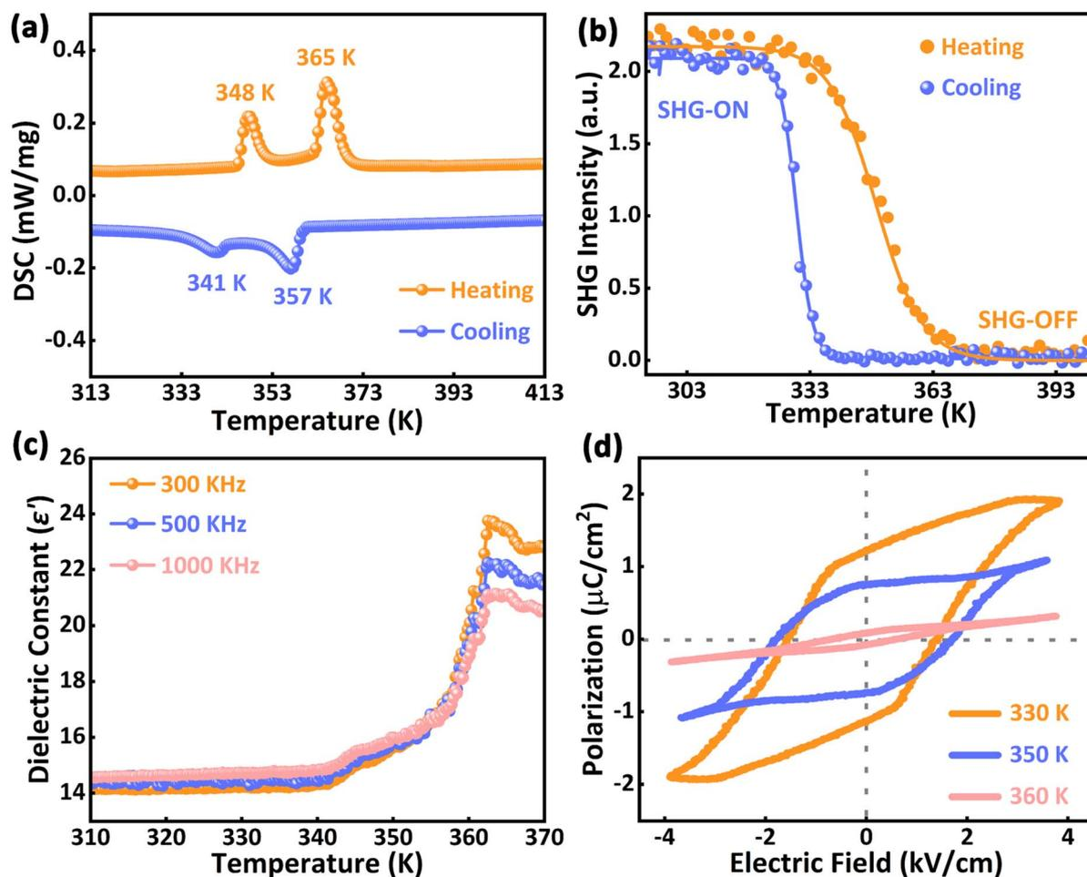
Fig. 2 Characterization of ferroelectricity of  $(Cl-PA)_2PbBr_4$ . (a) The phase transition behavior of  $(Cl-PA)_2PbBr_4$ . (b) The changes in SHG signals during the heating and cooling processes. (c) Variable-temperature dielectric measurements of  $(Cl-PA)_2PbBr_4$ . (d) Temperature-dependent variation of the  $P-E$  hysteresis loops of  $(Cl-PA)_2PbBr_4$ .
