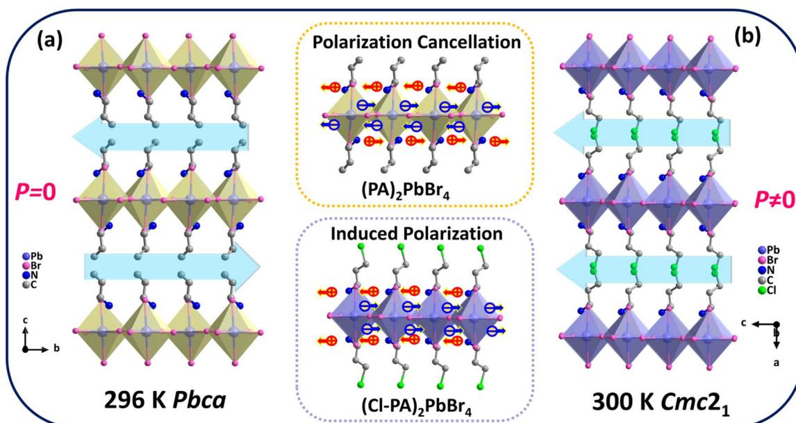
Fig. 1 The crystal structures of (PA)<sub>2</sub>PbBr<sub>4</sub> (a) and (Cl-PA)<sub>2</sub>PbBr<sub>4</sub> (b) at room temperature.
