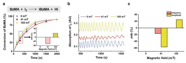
Fig. 2 MFEs on the conversion of BzMA. (a) Time trace of the BzMA conversion measured by HPLC at 0 mT (blue line), 41 mT (red line), and 100 mT (green line). (b) Time trace of I<sub>2</sub> absorbance (460 nm) in BzMA oscillating systems at 0, 41, and 100 mT. (c) Comparison of mfe between frequency and amplitude in Fig. 2b.
