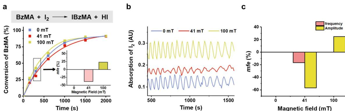
Fig. 2 MFEs on the conversion of BzMA. (a) Time trace of the BzMA conversion measured by HPLC at 0 mT (blue line), 41 mT (red line), and 100 mT (green line). (b) Time trace of  $I_2$  absorbance (460 nm) in BzMA oscillating systems at 0, 41, and 100 mT. (c) Comparison of *mfe* between frequency and amplitude in Fig. 2b.
