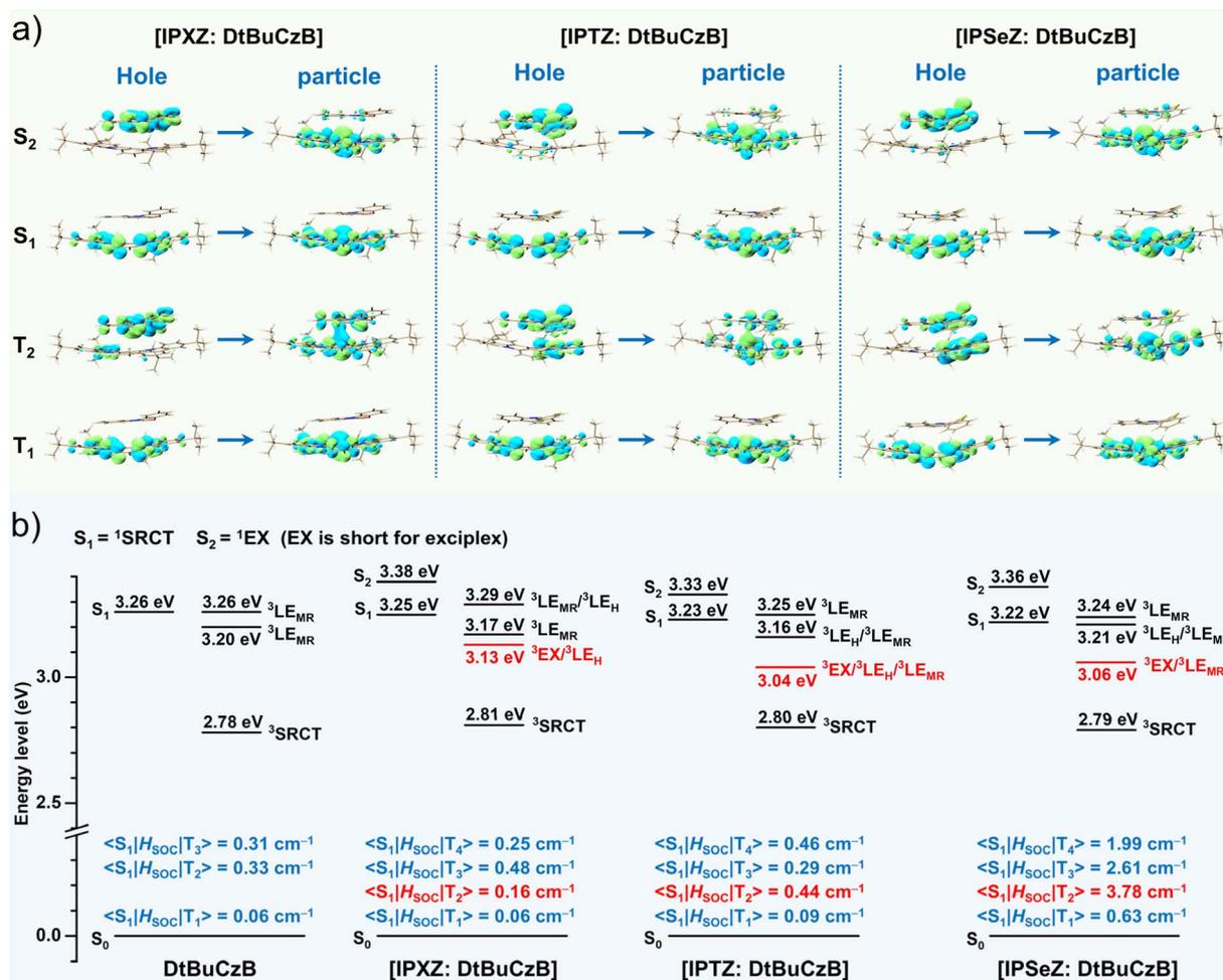
Fig. 2 (a) NTO analysis for the S<sub>1</sub>, S<sub>2</sub>, T<sub>1</sub> and T<sub>2</sub> states of the [host unit: DtBuCzB] combination. (b) Excited-state energy levels and SOCMEs between the S<sub>1</sub> and low-lying triplet states.
