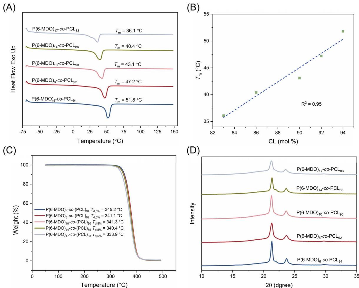
Fig. 3 (A) DSC traces of P(6-MDO)-co-PCL with varied 6-MDO incorporations (6–17 mol%). (B) Plot of the melting temperature ( $T_m$ ) vs. the composition. (C) TGA traces of P(6-MDO)-co-PCL with varied 6-MDO incorporations (6–17 mol%). (D) XRD traces of P(6-MDO)-co-PCL with varied 6-MDO incorporations (6–17 mol%).
