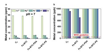
Fig. 4 (a) Batch adsorption experiments in Cr(vi) spiked river water at pH 7, adsorption dosage of 0.5 g  $L^{-1}$ , and an initial Cr concentration of 900 ppb; (b) zoomed in view of (a) showing low metal concentrations. The red dashed line indicates the WHO limit for chromium.
