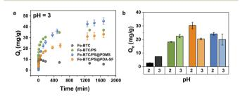
Fig. 2 (a) The extraction of Cr(vi) species plotted as a function of time by Fe-BTC, Fe-BTC/PS, Fe-BTC/PS@PDA-SF, and Fe-BTC/PS@PDMS from aqueous acidic media (pH 3); (b) Cr(vi) batch adsorption experiments at pH 2 and 3 for Fe-BTC (black), Fe-BTC/PS (green), Fe-BTC/PS@PDA-SF (orange) and Fe-BTC/PS@PDMS (blue).
