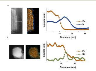
Fig. 3 HAADF-STEM images and corresponding EDX elemental maps (left) and line scans (right) from a sliced crystallite of (a) Fe-BTC/PS@PDA-SF and (b) Fe-BTC/PS@PDMS.
